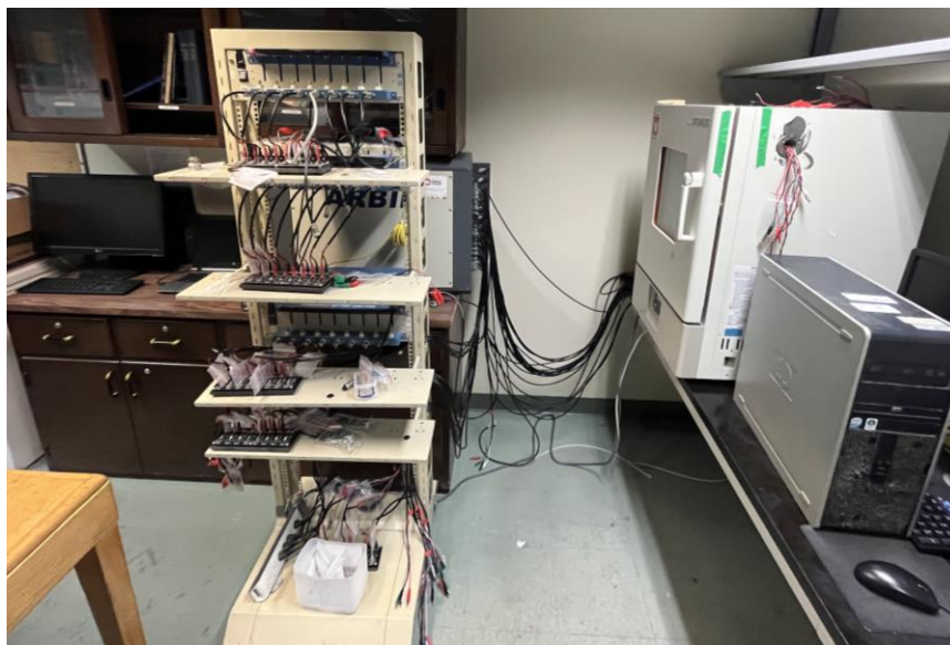
Figure 3. 4. The MTI battery tester (BST8-WA, MTI corporation) employed for battery cycling tests, including plating-stripping and charge-discharge cycling.
