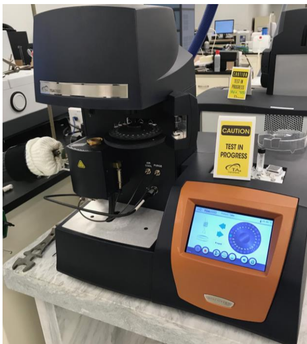
Figure 3. 10. The thermogravimetric analysis (TGA) Discovery 5500 from TA Instruments.
