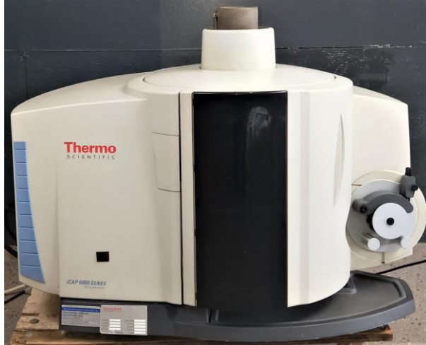
Figure 3. 13. The inductively coupled plasma optical emission spectroscopy (ICP-OES, Thermo Scientific iCAP 6500 ICP spectrometer).
