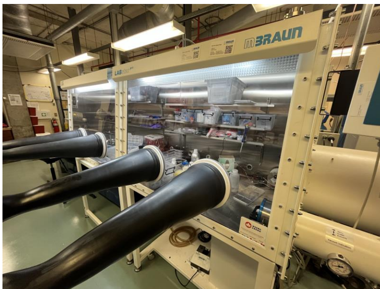
Figure 3. 3. The Argon-filled glovebox utilized for battery assembling and material preparation.
