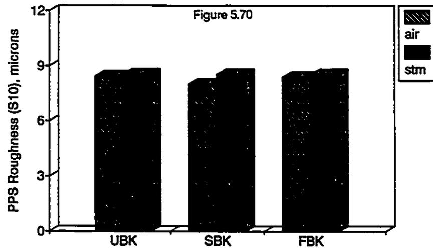
Figures 5.69 - 5.70: Effect of Bleaching and Drying Fluid on Viscosity and PPS Roughness
