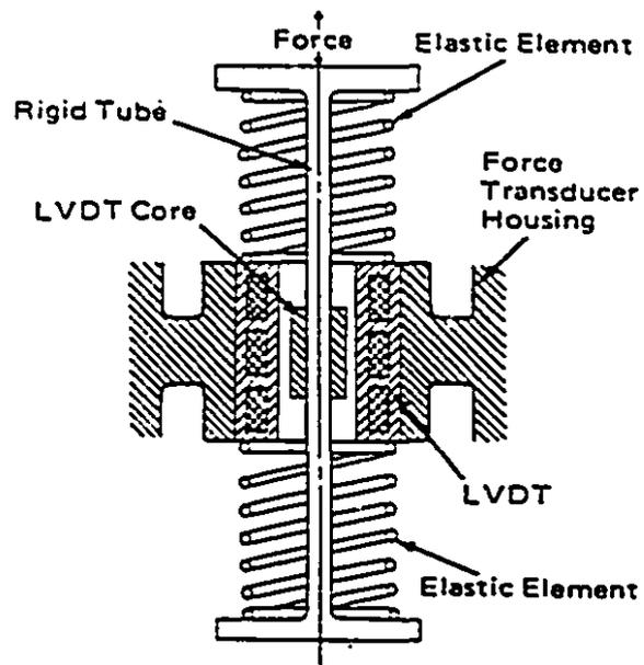
Figure 3.3b: Internal view of load cell
