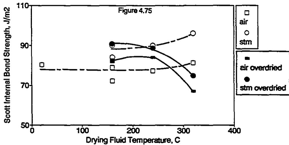
Figures 4.73 - 4.75: Effect of Drying Fluid and Temperature on Fold, Zero-Span Breaking Length and Scott Internal Bond Strength
