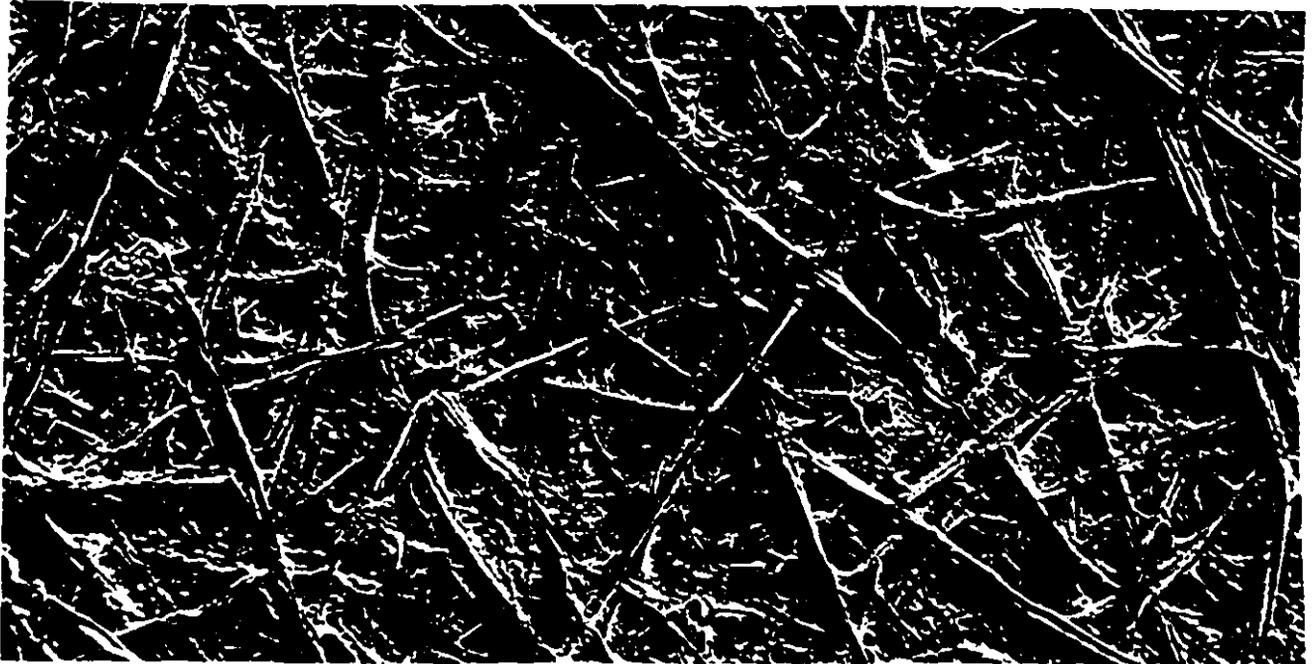
Figure 4.23a: Scanning Electron Micrograph of Steam Dried TMP sheet surface
