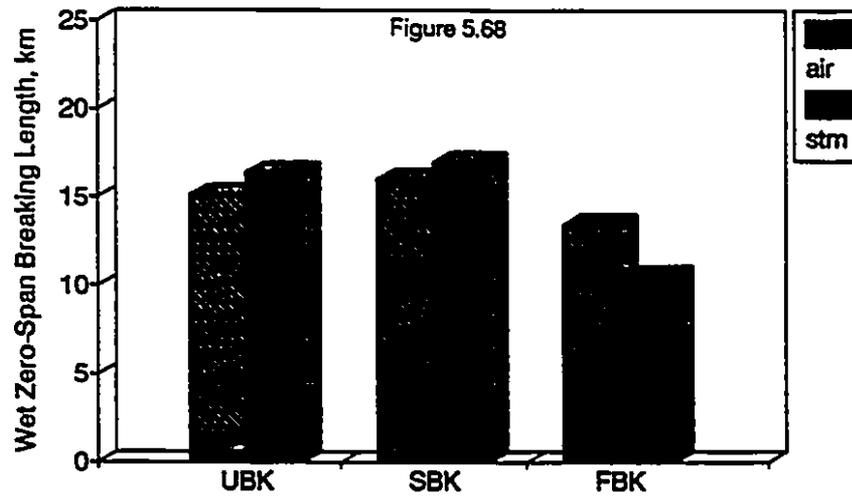
Figures 5.67 - 5.68: Effect of Bleaching and Drying Fluid on Zero-Span Breaking Length and Wet Zero-Span Breaking Length
