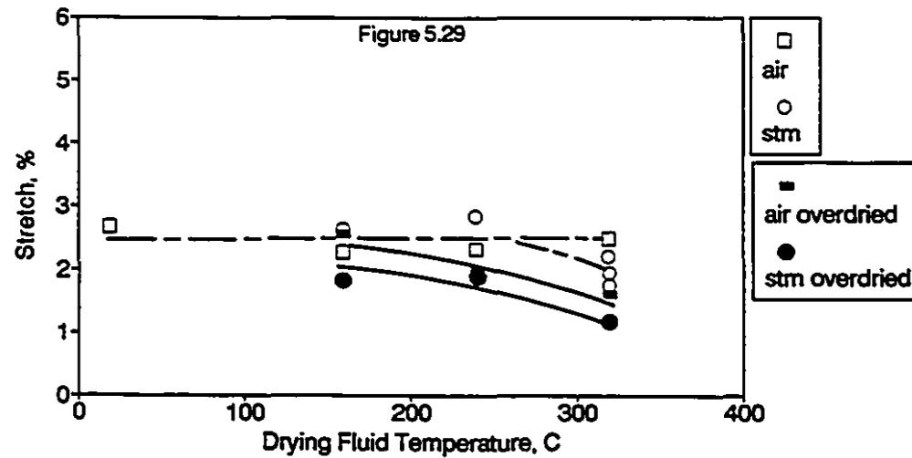
Figures 5.27 - 5.29: Effect of Drying Fluid and Temperature on Fold, Tensile Index and Stretch
