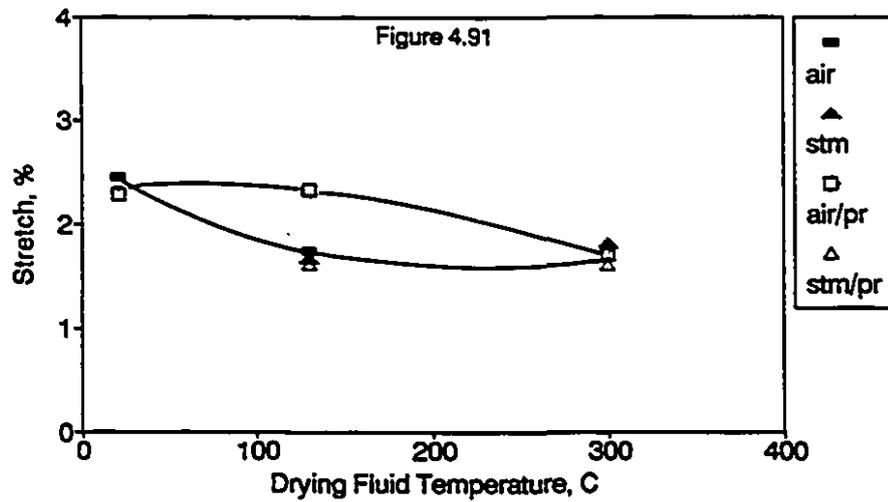
Figures 4.90 - 4.91: Effect of Drying Fluid, Temperature and Pressing on Fold and Stretch
