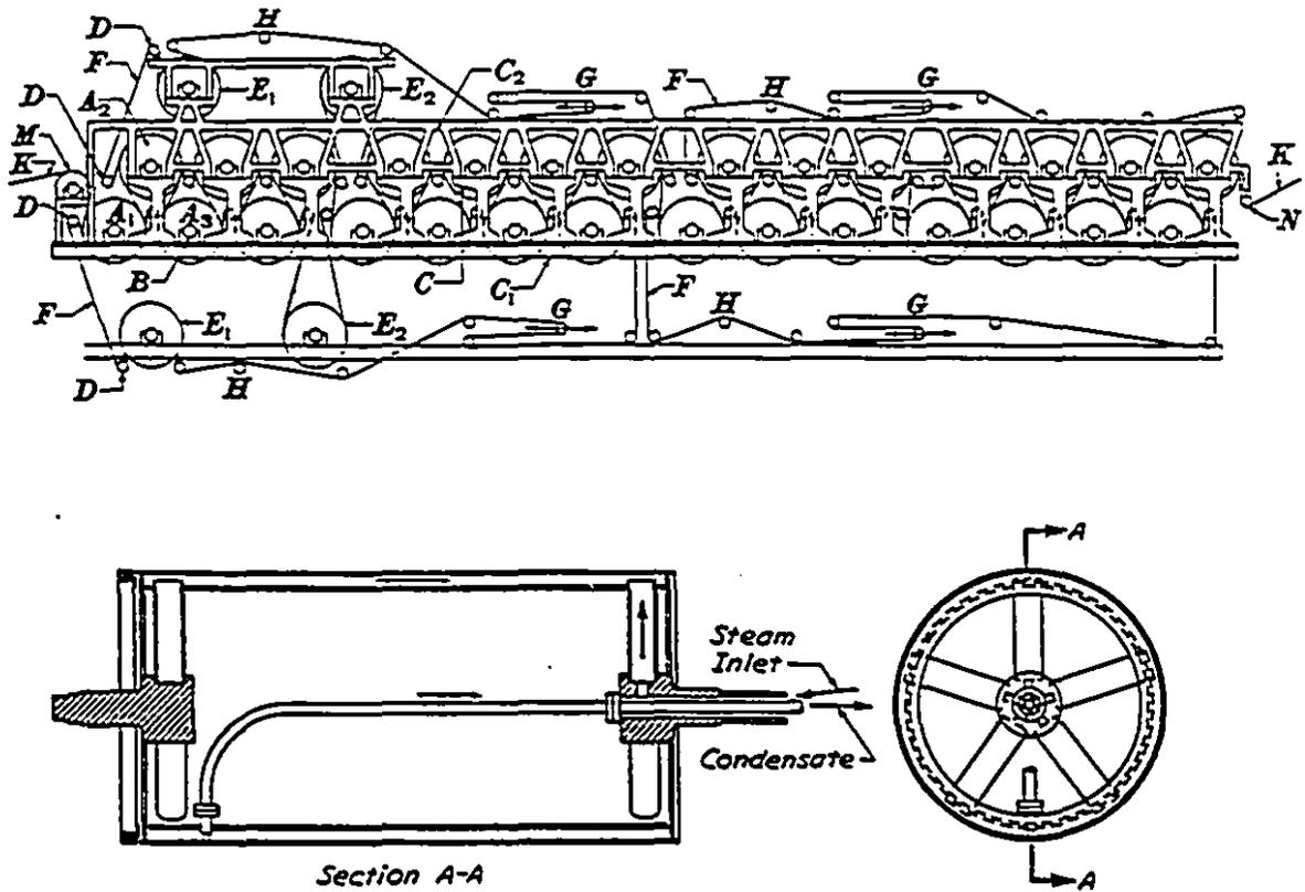
Figure 1.1: Conventional dryer section
