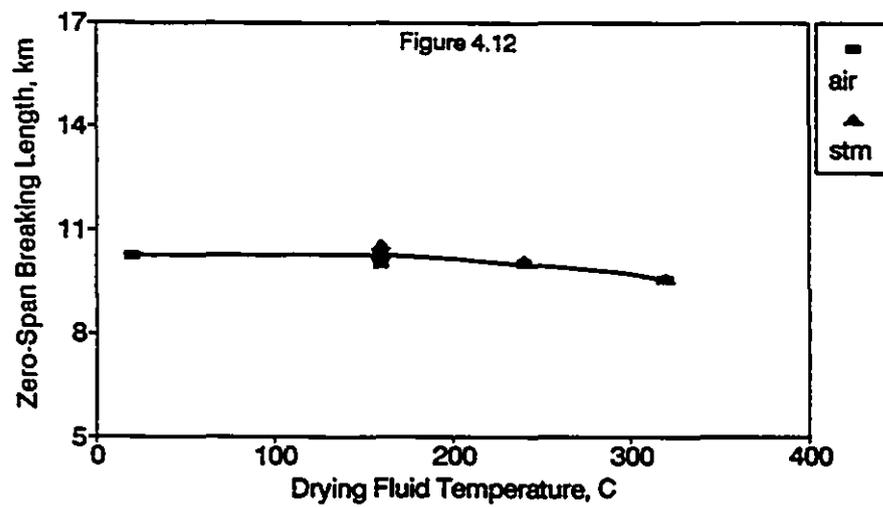
Figures 4.10 - 4.12: Effect of Drying Fluid and Temperature on Tear Index, Fold and Zero-Span Breaking Length
