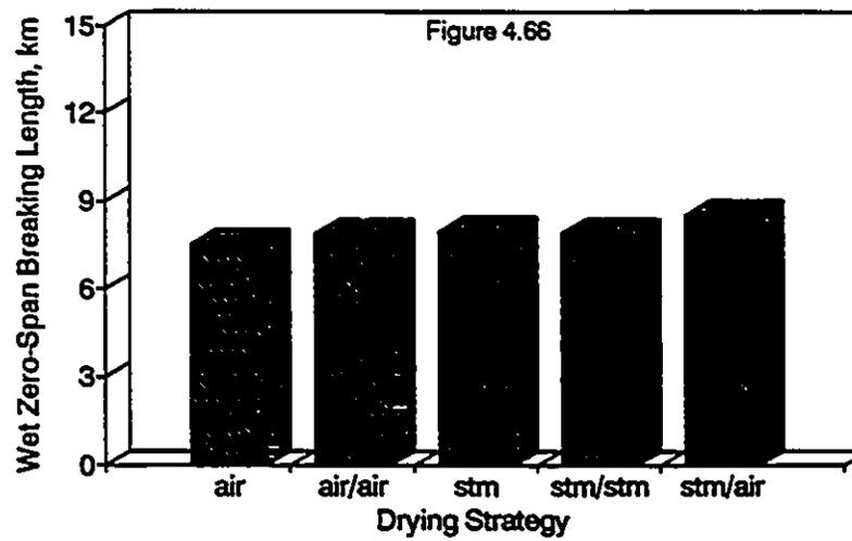
Figures 4.65 - 4.66: Effect of Recycling and Drying Fluid on Zero-Span Breaking Length and Wet Zero-Span Breaking Length
