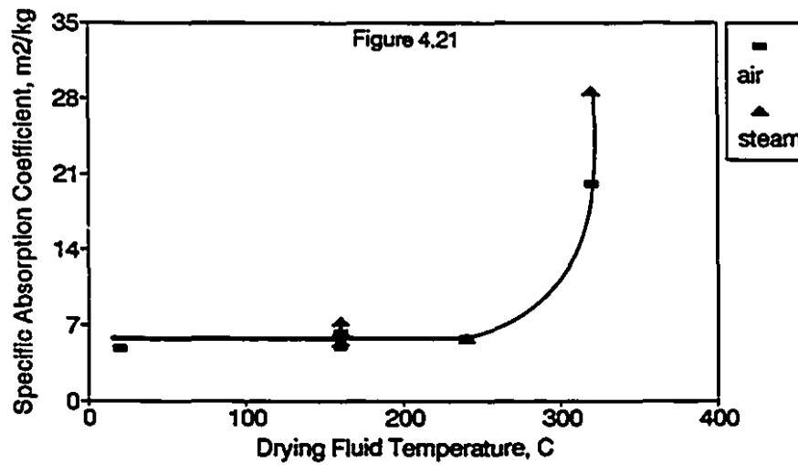
Figures 4.19 - 4.21: Effect of Drying Fluid and Temperature on Brightness, Opacity and Specific Absorption Coefficient
