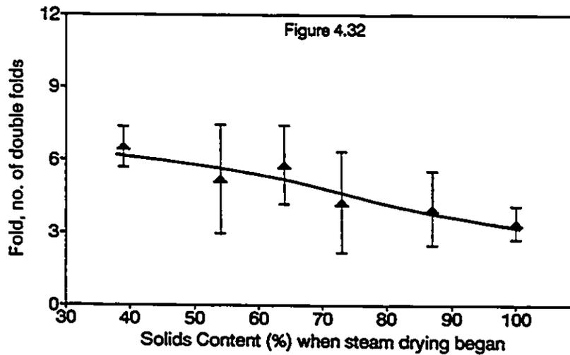
Figures 4.30 - 4.32: Effect of Initial Sheet Solids Content on Tensile Index, Tensile Energy Absorption Index and Fold
