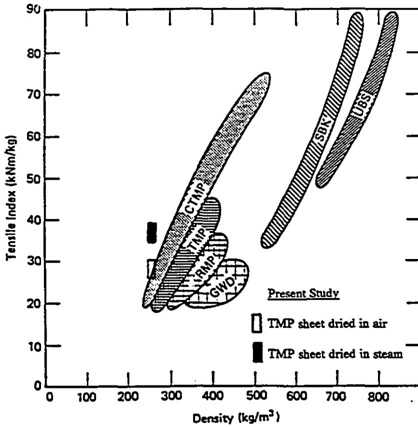
Figure 4.92: Relation between Tensile Index and Density for Various Pulp
