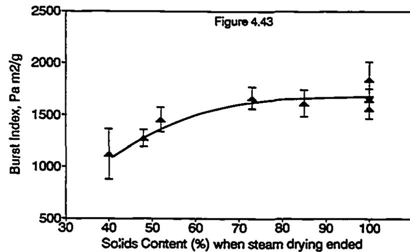
Figures 4.41 - 4.43: Effect of Final Sheet Solids Content on Zero-Span Breaking Length, Wet Zero-Span Breaking Length and Burst Index
