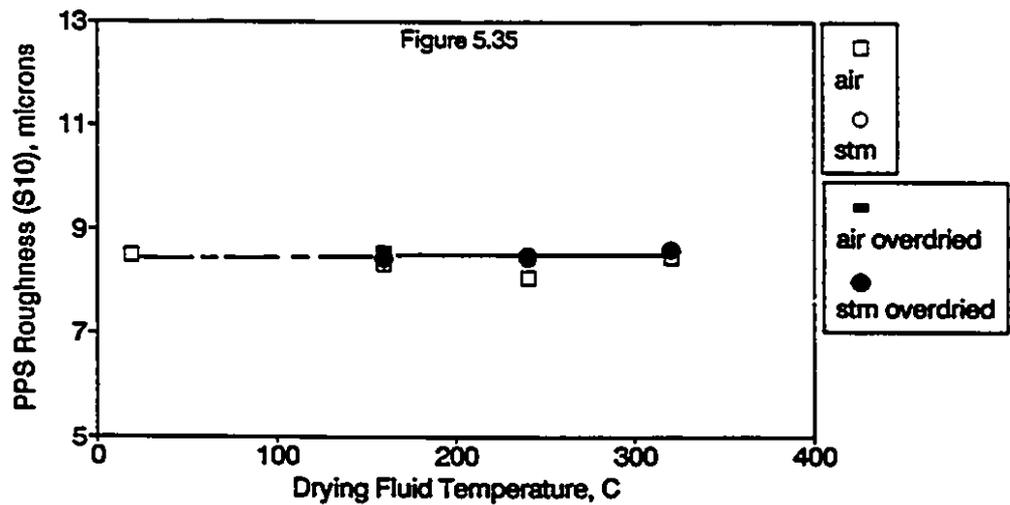
Figures 5.33 - 5.35: Effect of Drying Fluid and Temperature on Wet Zero-Span Breaking Length, Wet Tensile Strength and PPS Roughness
