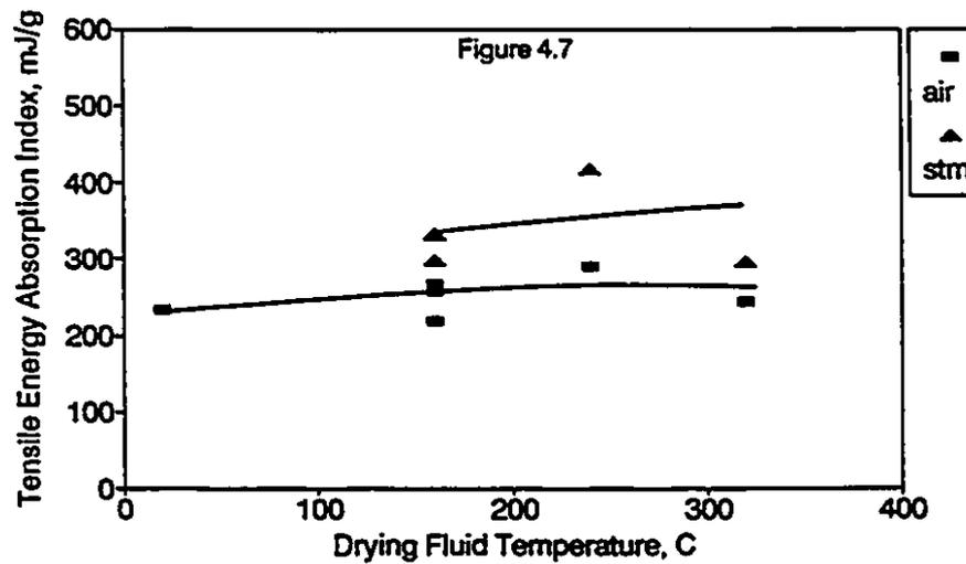
Figures 4.5 - 4.7: Effect of Drying Fluid and Temperature on Tensile Index, Stretch and Tensile Energy Absorption Index
