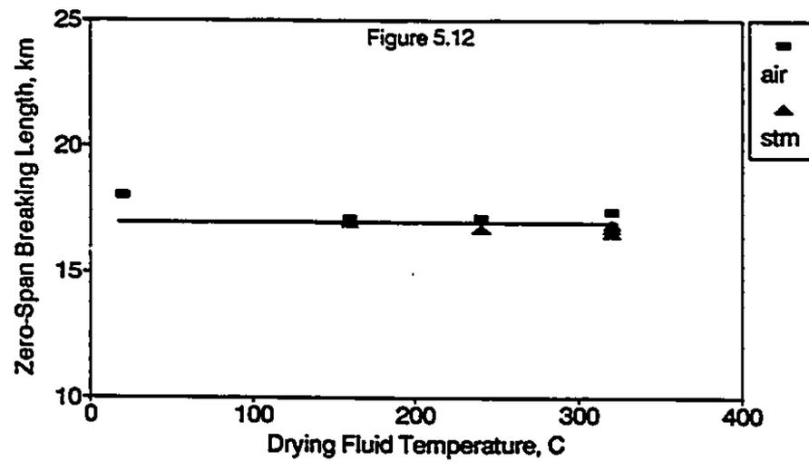
Figures 5.10 - 5.12: Effect of Drying Fluid and Temperature on Stretch, Tensile Energy Absorption Index and Zero-Span Breaking Length
