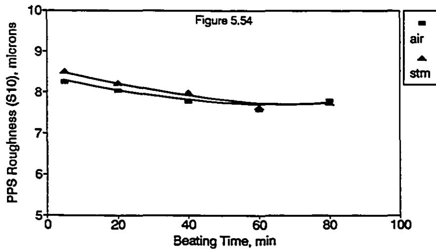
Figures 5.52 - 5.54: Effect of Beating Time and Drying Fluid on Zero-Span Breaking Length, Wet Zero-Span Breaking Length and PPS Roughness
