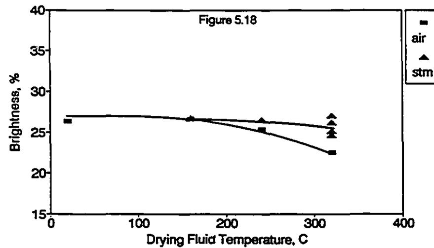
Figures 5.16 - 5.18: Effect of Drying Fluid and Temperature on Water Drop Absorption Time, PPS Roughness and Brightness
