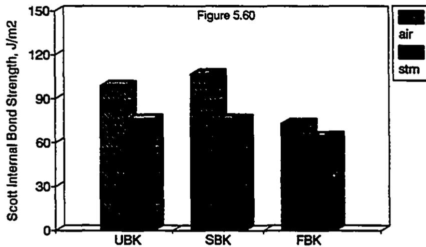
Figures 5.58 - 5.60: Effect of Bleaching and Drying Fluid on Tensile Index, Tensile Energy Absorption Index and Scott Internal Bond Strength
