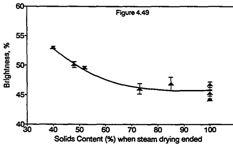
Figure 4.47 - 4.49: Effect of Final Sheet Solids Content on Fold, Scott Internal Bond Strength and Brightness
