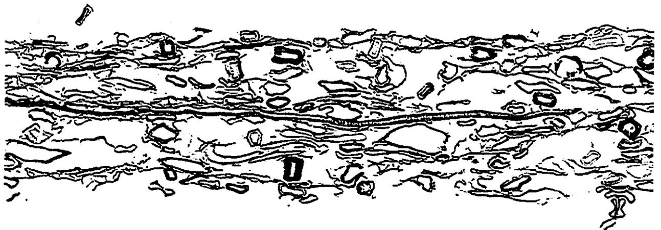
Figure 4.23d: SEM cross-sectional view of air dried TMP sheet (mag. X 200)
