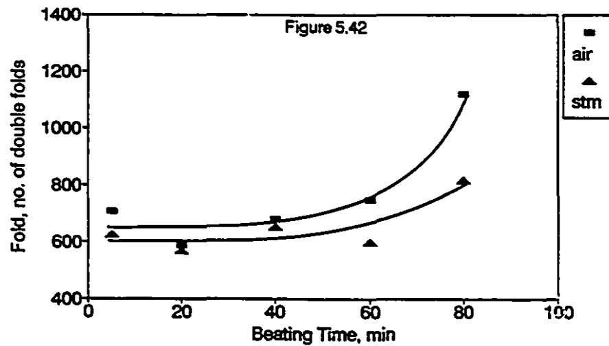
Figures 5.40 - 5.42: Effect of Beating Time and Drying Fluid on Bulk, Burst Index and Fold
