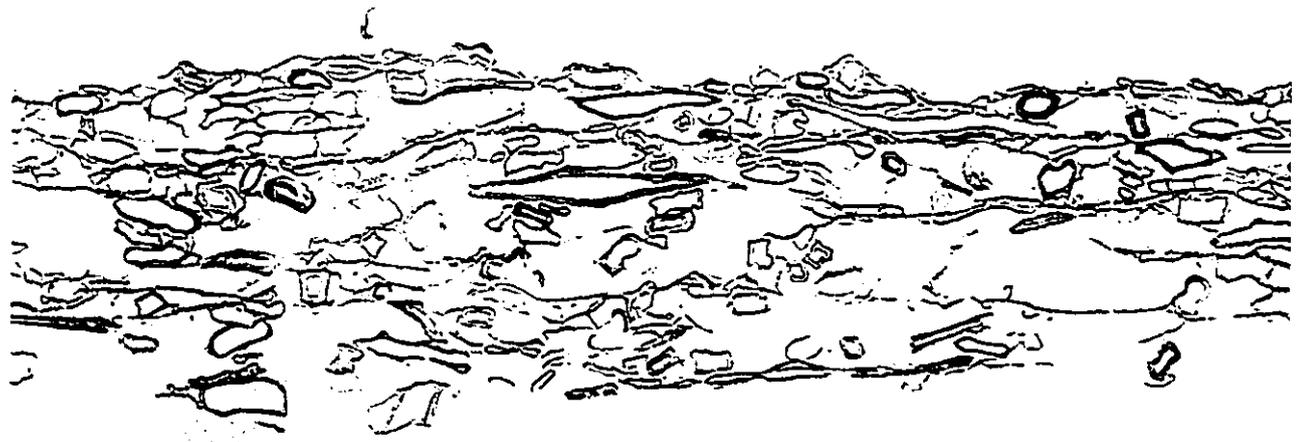
Figure 4.23c: SEM cross-sectional view of steam dried TMP sheet (mag. X 200)
