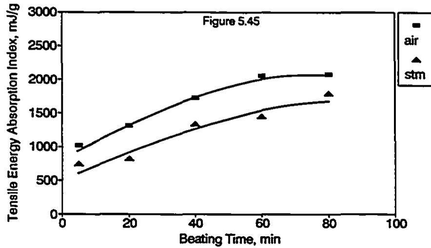
Figures 5.43 - 5.45: Effect of Beating Time and Drying Fluid on Tensile Index, Stretch and Tensile Energy Absorption Index
