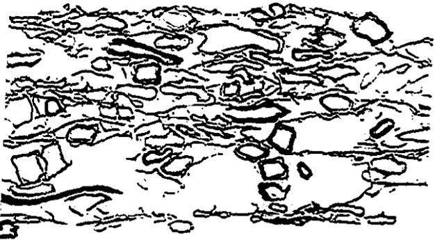
Further evidence of this is the diminished rugosity of the fibre contours which are covered with a film of softened fines material. No fibre collapse is observable. The increased roughness of the steam dried sheet surface is also evident. The micrographs thus serve as further proof for the hypothesis that it is mainly the fines fraction which is plasticized by the higher temperatures reached in superheated steam drying.
