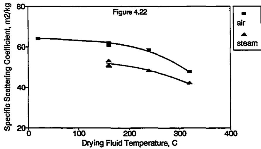
Figure 4.22: Effect of Drying Fluid Temperature on Specific Scattering Coefficient
