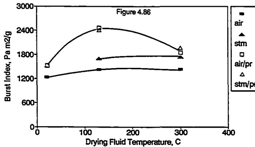
Figures 4.84 - 4.86: Effect of Drying Fluid, Temperature and Pressing on Bulk Standard Deviation, Bulk and Burst Index
