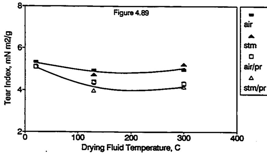
Figures 4.87 - 4.89: Effect of Drying Fluid, Temperature and Pressing on Tensile Index, Tensile Energy Absorption Index and Tear Index
