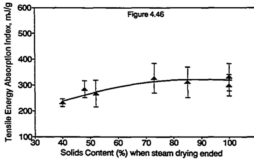
Figures 4.44 - 4.46: Effect of Final Sheet Solids Content on Tensile Index, Elastic Modulus and Tensile Energy Absorption Index
