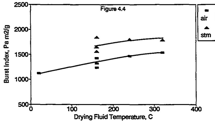
Figures 4.2 - 4.4: Effect of Drying Fluid and Temperature on Bulk, PPS Roughness and Burst Index
