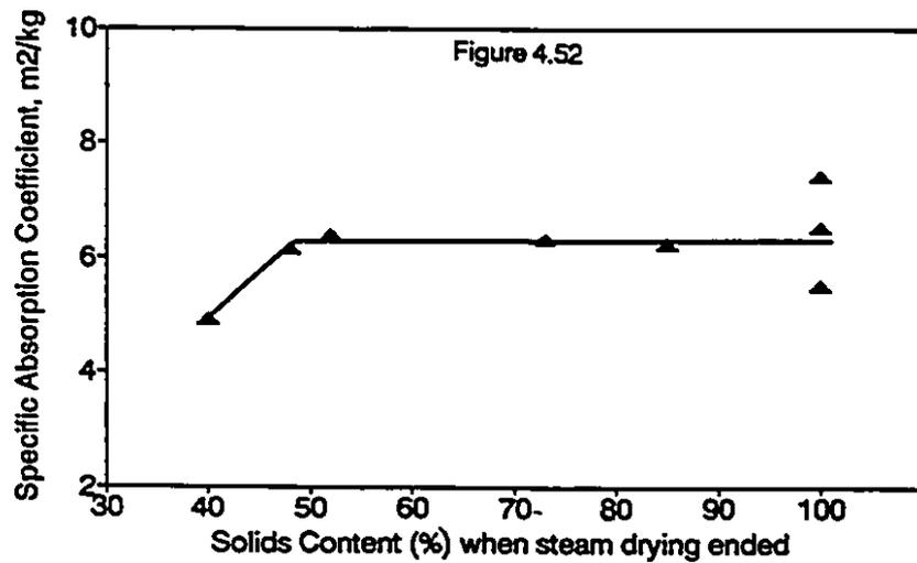
Figures 4.50 - 4.52: Effect of Final Sheet Solids Content on Specific Scattering Coefficient, Opacity and Specific Absorption Coefficient
