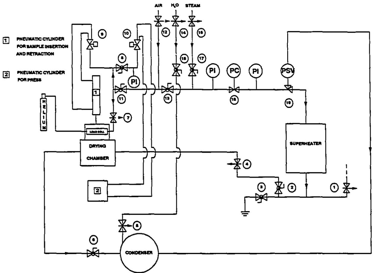
Figure 3.6: Schematic diagram of drying apparatus piping system
