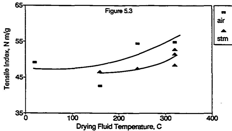
Figures 5.1 - 5.3: Effect of Drying Fluid and Temperature on Bulk, Burst Index and Tensile Index
