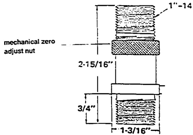
Figure 3.3a: External view of load cell
