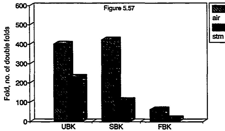
Figures 5.55 - 5.57: Effect of Bleaching and Drying Fluid on Bulk, Burst Index and Fold
