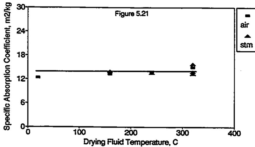
Figures 5.19 - 5.21: Effect of Drying Fluid and Temperature on Opacity, Specific Scattering Coefficient and Specific Absorption Coefficient
