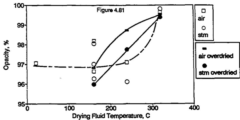
Figures 4.79 - 4.81: Effect of Drying Fluid and Temperature on PPS Roughness, Brightness and Opacity
