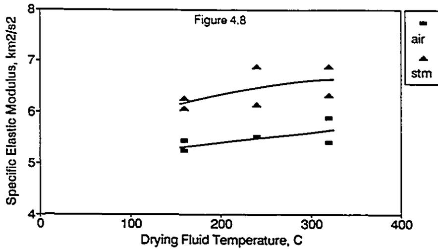
Figure 4.8: Effect of Drying Fluid and Temperature on Elastic Modulus
