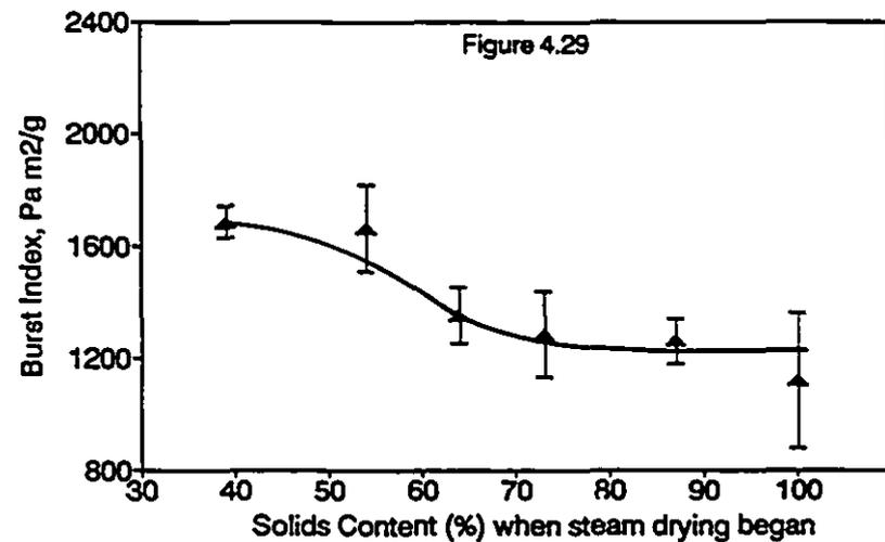
Figures 4.27 - 4.29: Effect of Initial Sheet Solids Content on Zero-Span Breaking Length, Wet Zero-Span Breaking Length and Burst Index
