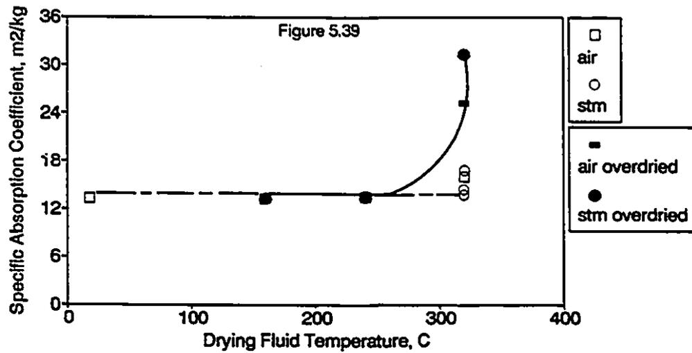
Figures 5.38 - 5.39: Effect of Drying Fluid and Temperature on Specific Scattering Coefficient and Specific Absorption Coefficient
