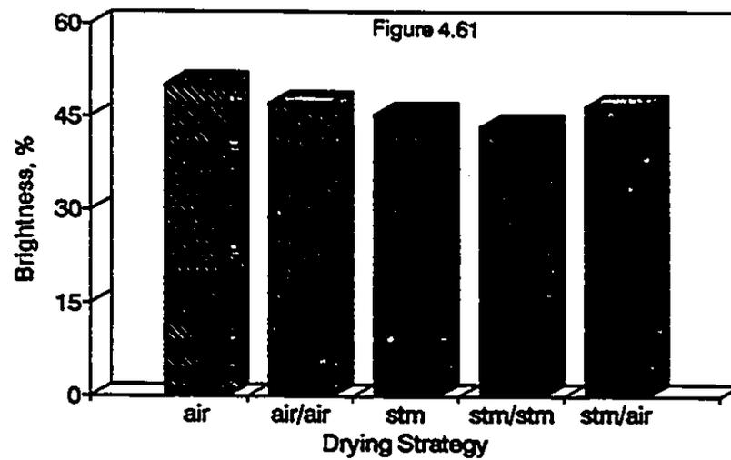
Figures 4.59 - 4.61: Effect of Recycling and Drying Fluid on Scott Internal Bond Strength, Stretch and Brightness
