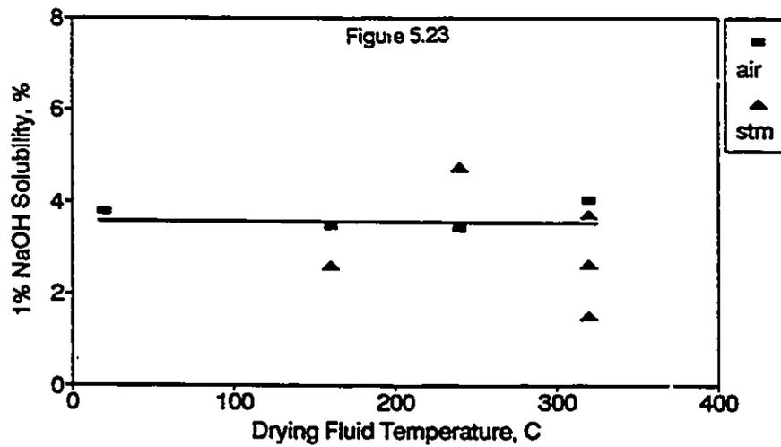
Figures 5.22 - 5.23: Effect of Drying Fluid and Temperature Viscosity and 1% NaOH Solubility
