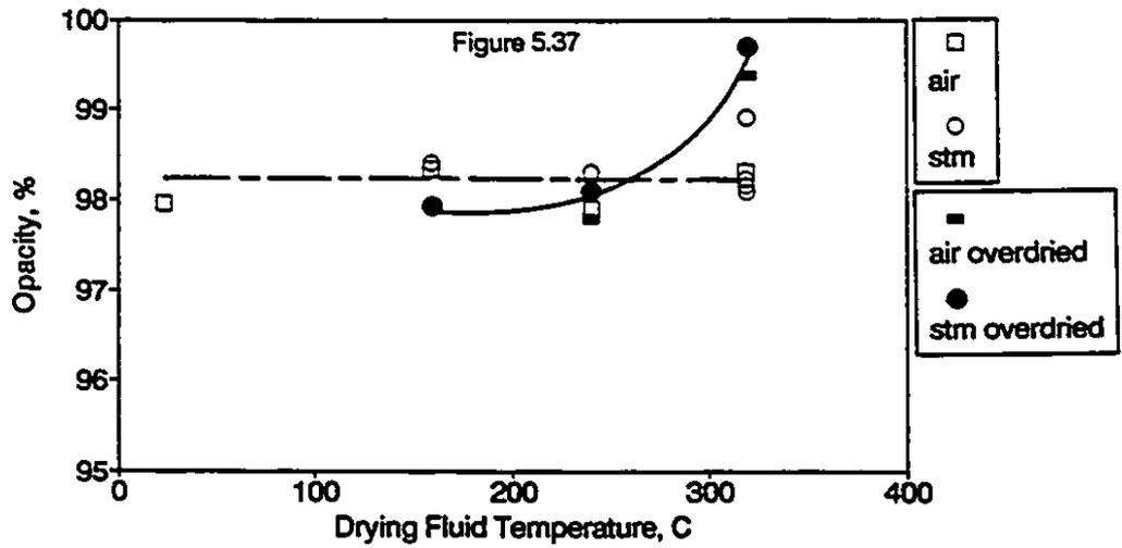
Figures 5.36 - 5.37: Effect of Drying Fluid and Temperature on Brightness and Opacity
