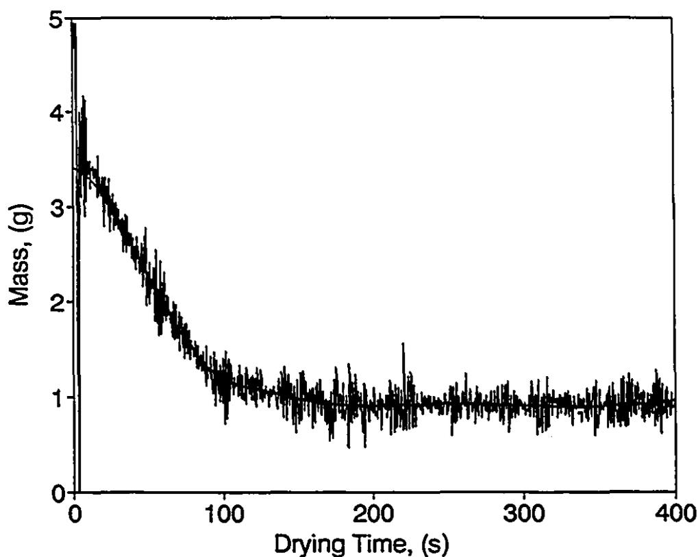
Figure 3.9: Effect of drying time on sheet mass for TMP sheet in 160°C steam
