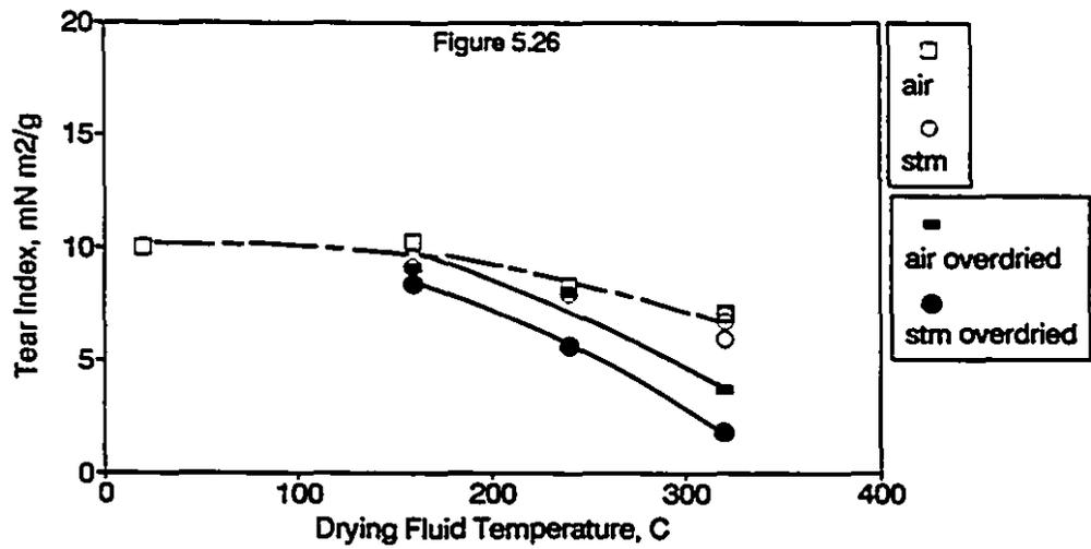
Figures 5.24 - 5.26: Effect of Drying Fluid and Temperature on Bulk, Burst Index and Tear Index
