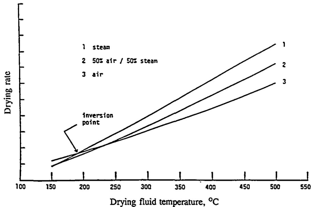
Figure 1.2: Evaporation rates for various free stream fluids
