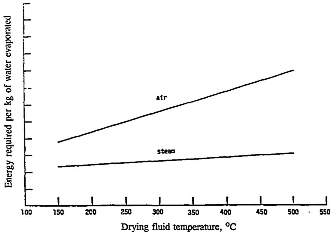
Figure 1.3: Effect of drying temperature on energy required for air and steam drying
