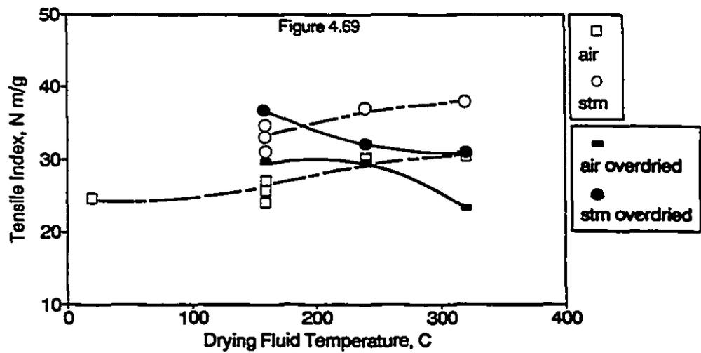
Figures 4.67 - 4.69: Effect of Drying Fluid and Temperature on Bulk, Burst Index and Tensile Index
