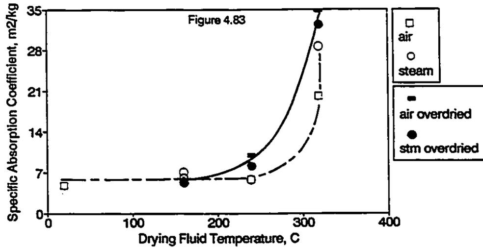
Figures 4.82 - 4.83: Effect of Drying Fluid and Temperature on Specific Scattering Coefficient and Specific Absorption Coefficient
