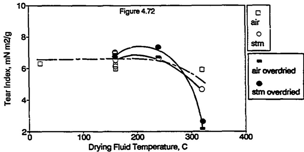
Figures 4.70 - 4.72: Effect of Drying Fluid and Temperature on Tensile Energy Absorption Index, Stretch and Tear Index
