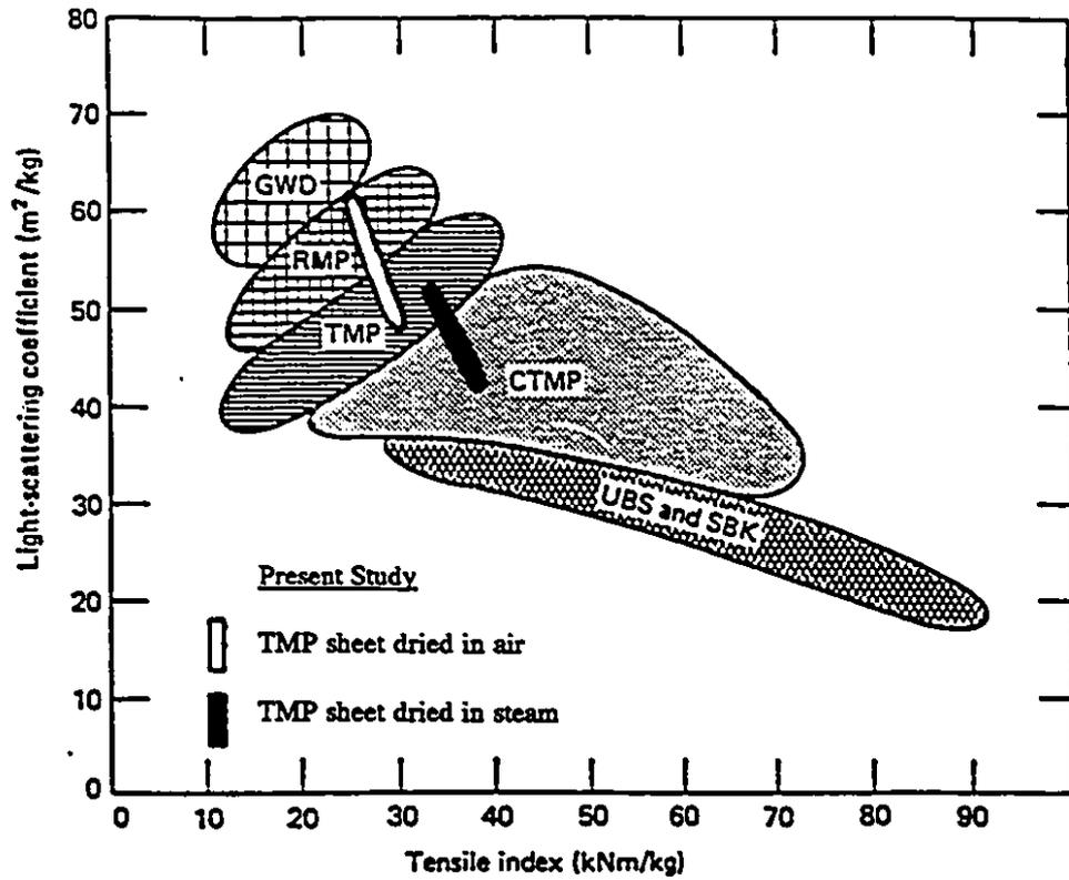
Figure 4.93: Relation between Light Scattering Coefficient and Tensile Index for Various Pulp
