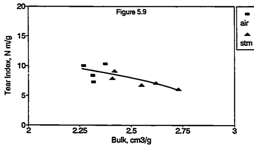
Figure 5.7 - 5.9: Effect of Bulk on Tensile Index, Fold and Tear Index
