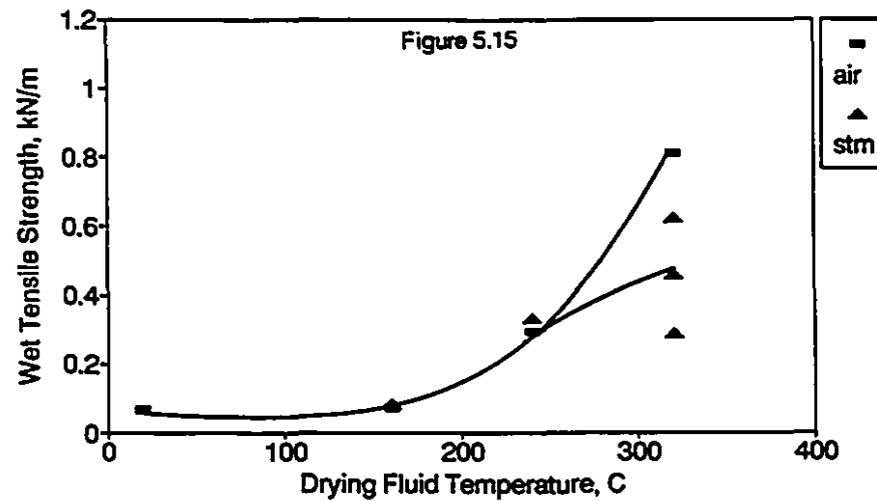
Figures 5.13 - 5.15: Effect of Drying Fluid and Temperature on Wet Zero-Span Breaking Length, Scott Internal Bond Strength and Wet Tensile Strength
