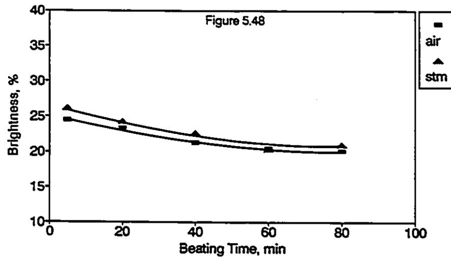
Figures 5.46 - 5.48: Effect of Beating Time and Drying Fluid on Scott Internal Bond Strength, Tear Index and Brightness
