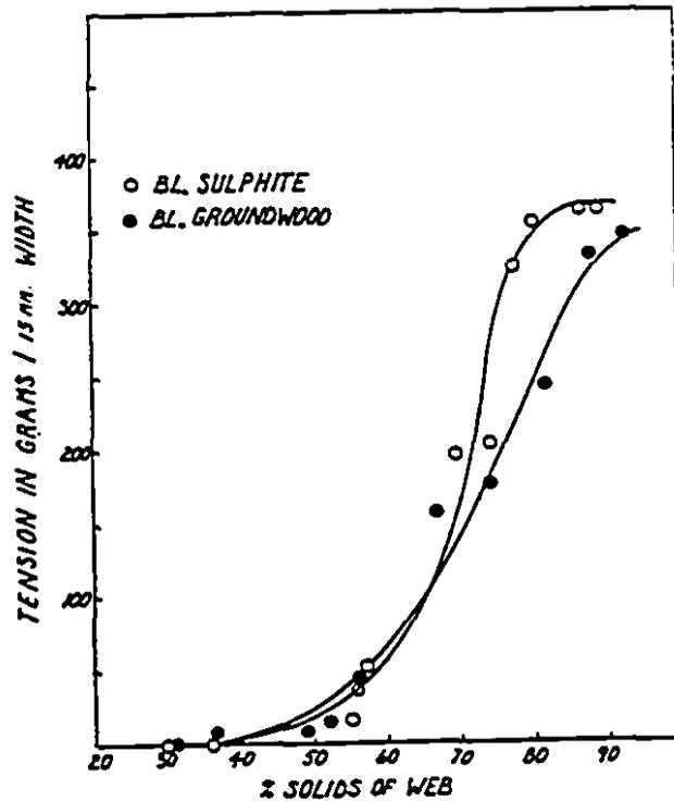
Figure 2.5: Evolution of drying force during restrained drying
