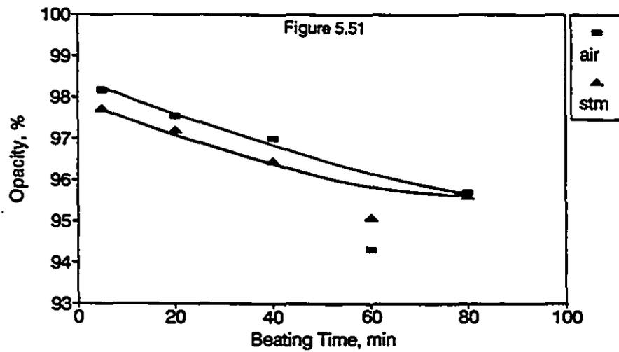
Figures 5.49 - 5.51: Effect of Beating Time and Drying Fluid on Specific Scattering Coefficient, Specific Absorption Coefficient and Opacity
