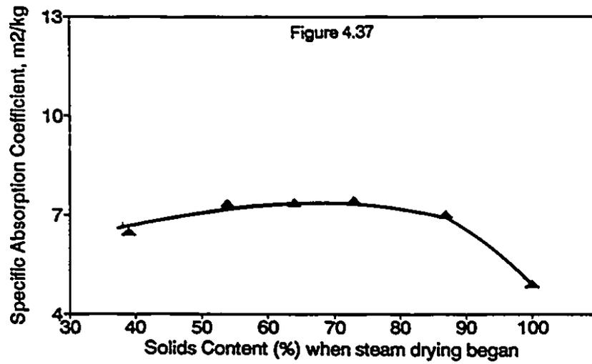
Figures 4.36 - 4.37: Effect of Initial Sheet Solids Content on Opacity and Specific Absorption Coefficient
