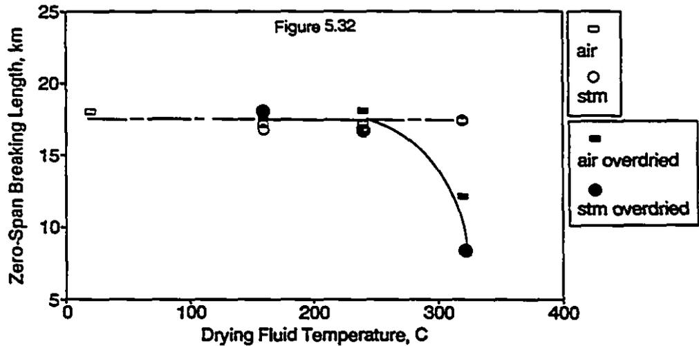
Figures 5.30 - 5.32: Effect of Drying Fluid and Temperature on Tensile Energy Absorption Index, Scott Internal Bond Strength and Zero-Span Breaking Length
