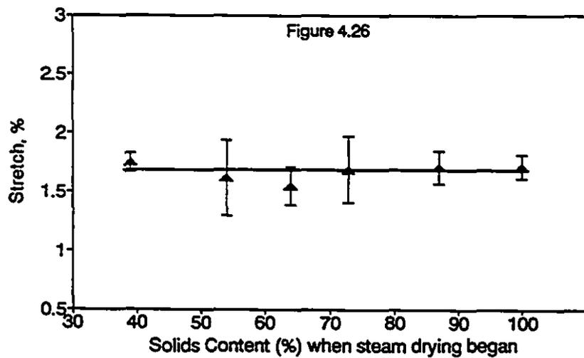
Figures 4.24 - 4.26: Effect of Initial Sheet Solids Content on Bulk, Tear Index and Stretch
