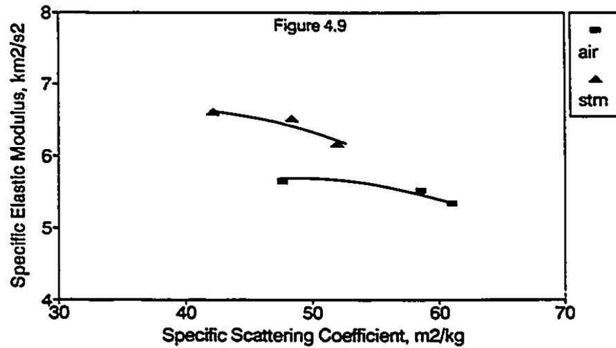
Figure 4.9: Effect of Scattering Coefficient and Drying Fluid on Elastic Modulus
