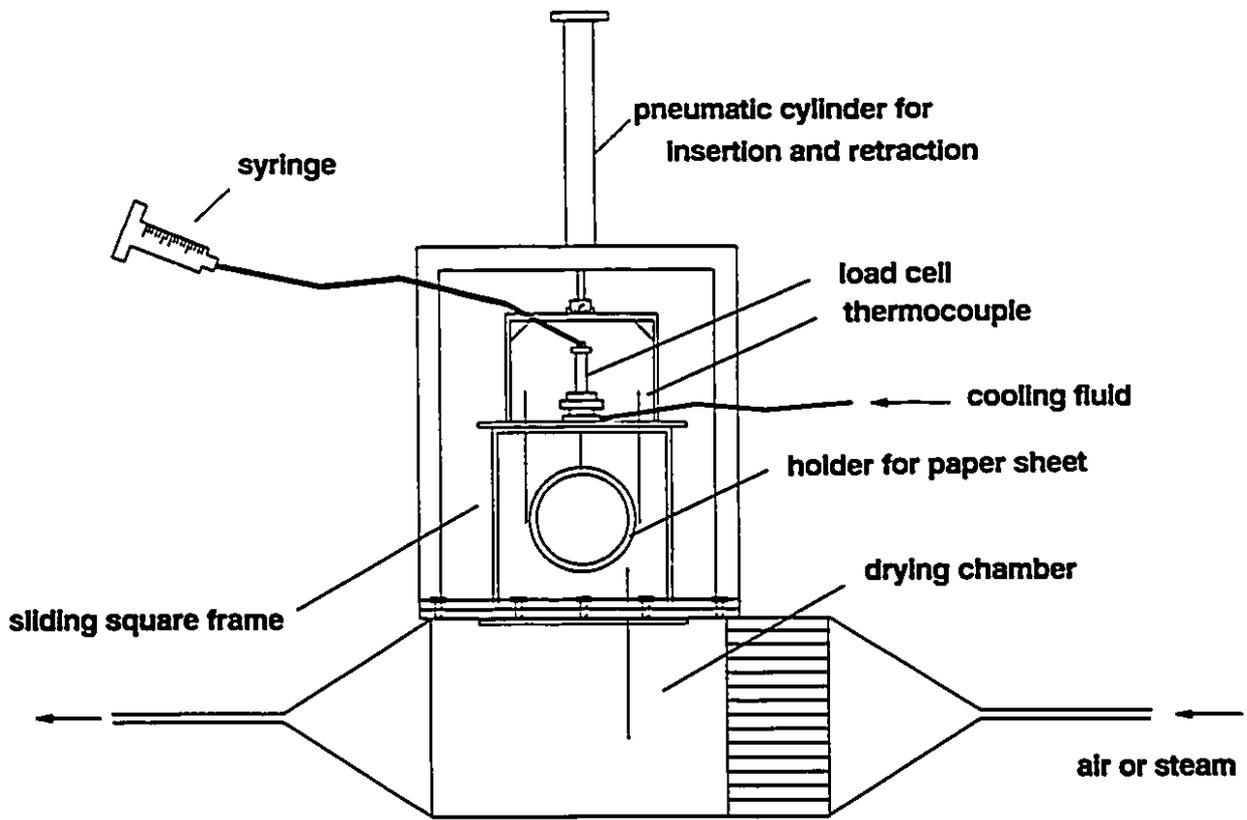
Figure 3.1: Schematic of drying apparatus
