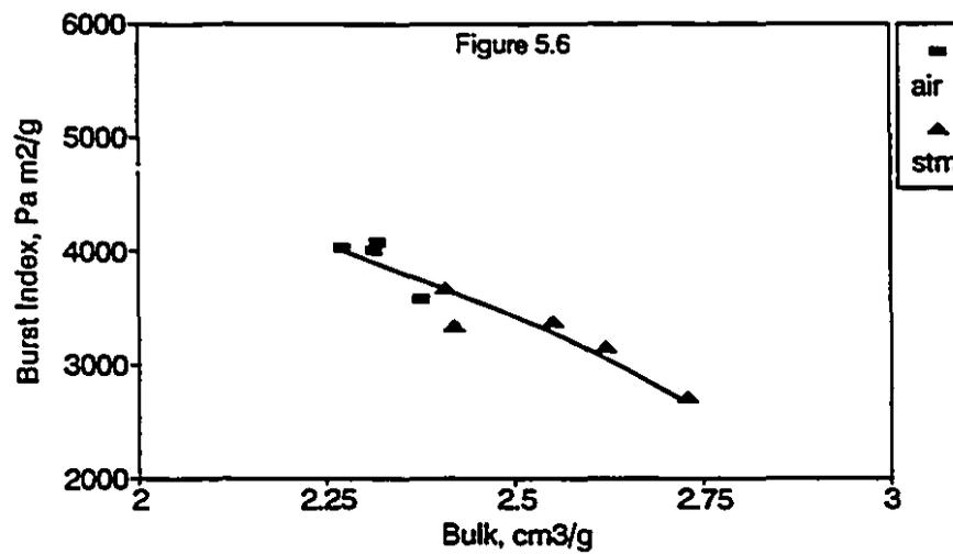
Figures 5.4 - 5.6: Effect of Drying Fluid and Temperature on Fold and Tear Index, Effect of Bulk on Burst Index
