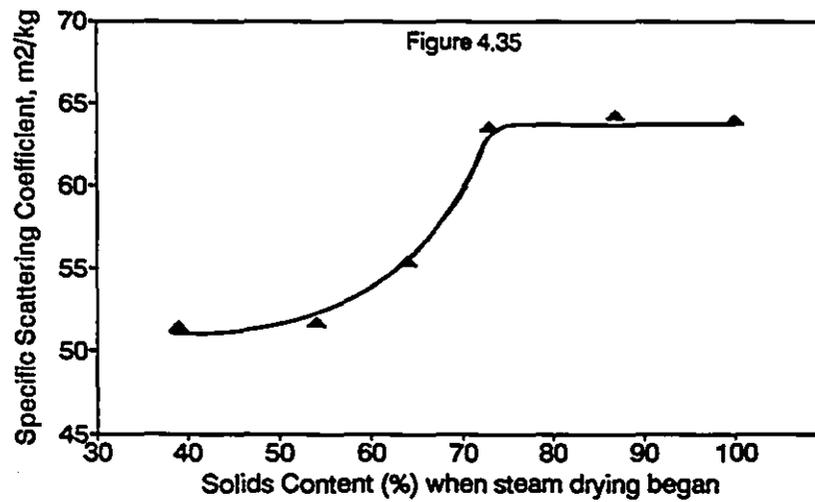
Figures 4.33 - 4.35: Effect of Initial Sheet Solids Content on Scott Internal Bond Strength, Brightness and Specific Scattering Coefficient
