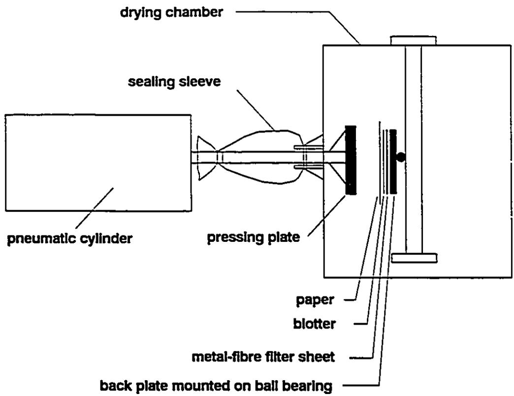
Figure 3.5: Schematic side view of press-drying arrangement
