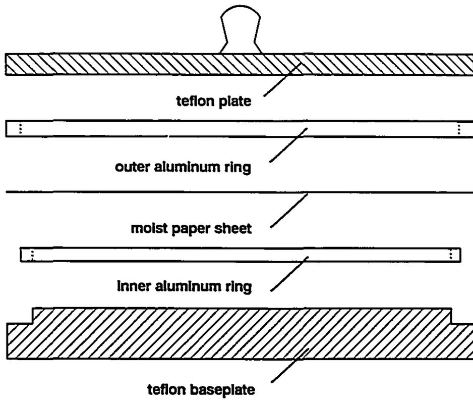
Figure 3.8: Paper holder: teflon baseplate and aluminum rings
