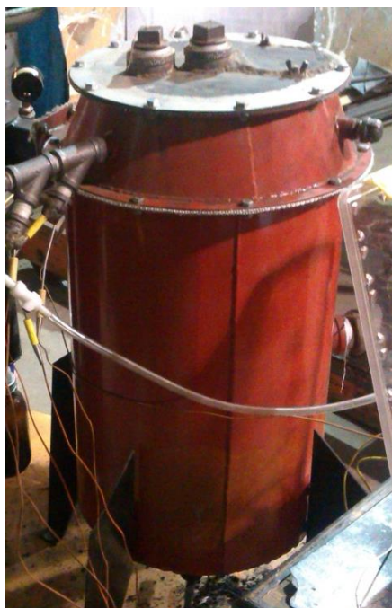
Figure 2.3. Pilot-scale GEK gasification reactor
