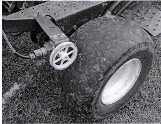
FIGURE 4.1. The encoder mounted on the mower in contact with the wheel.
