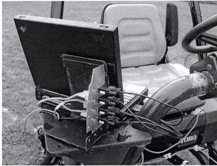
FIGURE 4.7. The screen support serves as the QSP-100 serial connectors holder.
