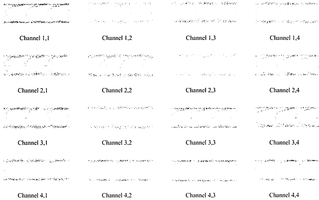
Figure 4.11 - System eye patterns generated from a 2^{23}-1 pseudo-random NRZ bit stream at 155Mb/s.
