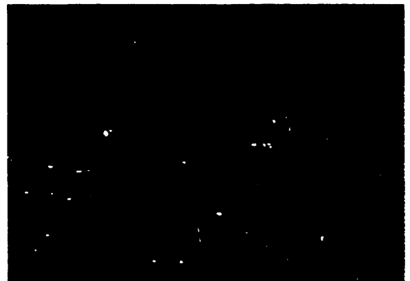
Figure 15. At 1 m/s fluid velocity, dispersed air bubbles exist at the top section of the image cell when it is configured horizontally
