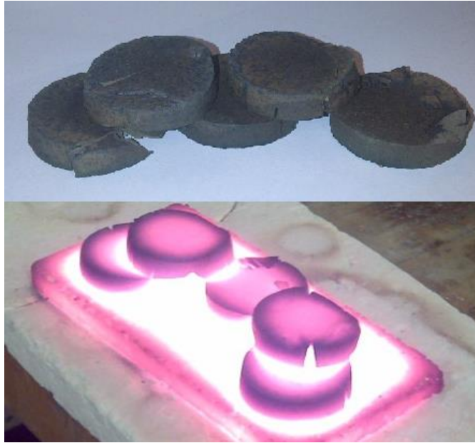
Figure 4 Eco-cement disks for clinkering
