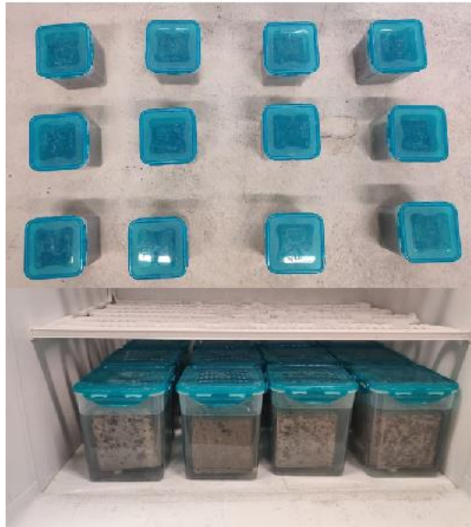
Figure 16 Thawing (top) and freezing (bottom) set up
