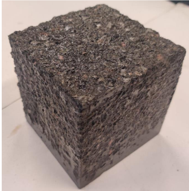
Figure 30 Typical concrete cube at 100 freeze/thaw cycles
