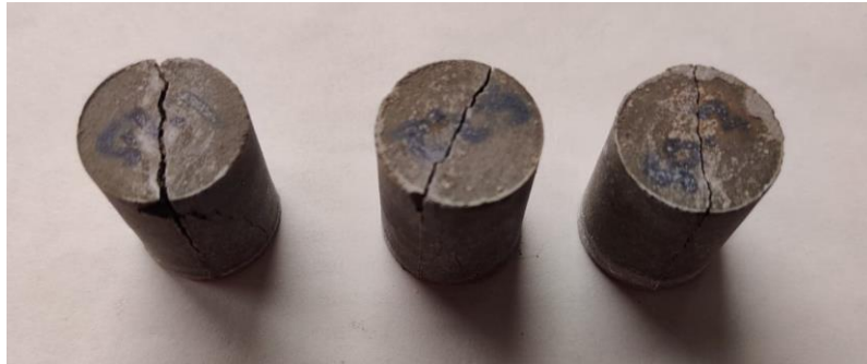
Figure 26 Cracking in 50%ECO paste samples
