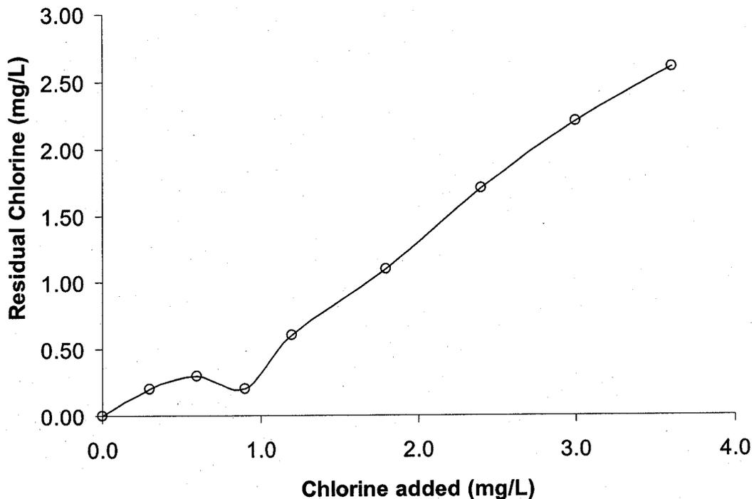
Figure 3.2. Chlorine demand curve for filtered water from Plant B.
