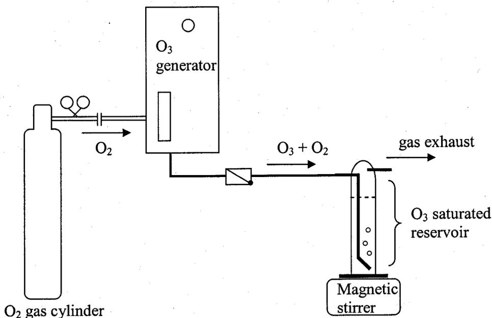
Figure 3.3. Diagram of ozone contacting apparatus.
