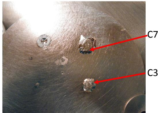
Figure 5-13: Plain view of underside of Ni target post evaporation of substrates C3( $ZrO_2$  and C7 ( $Al_2O_3$ )
