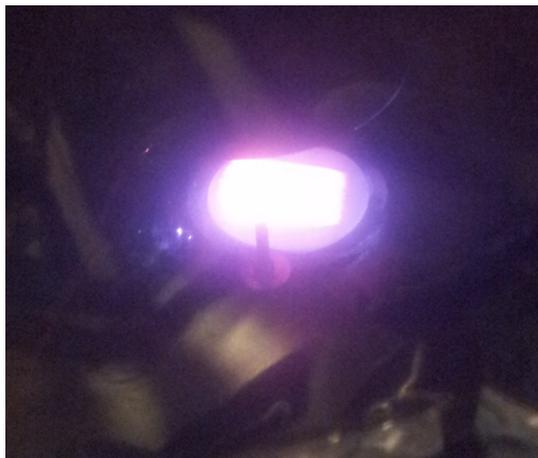
Figure 5-14: Plain view of plasma formation due to electron beam charging using a defocused beam on an  $\text{Al}_2\text{O}_3$  target. The color shown does not match the true color due to CCD distortion.
