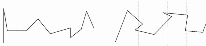
Figure 6.18: Left: An x -monotone chain. Right: A chain that is not x -monotone.
