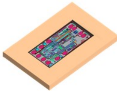
Figure 14-3: CMOS die mold with the CMOS die inside the mold
