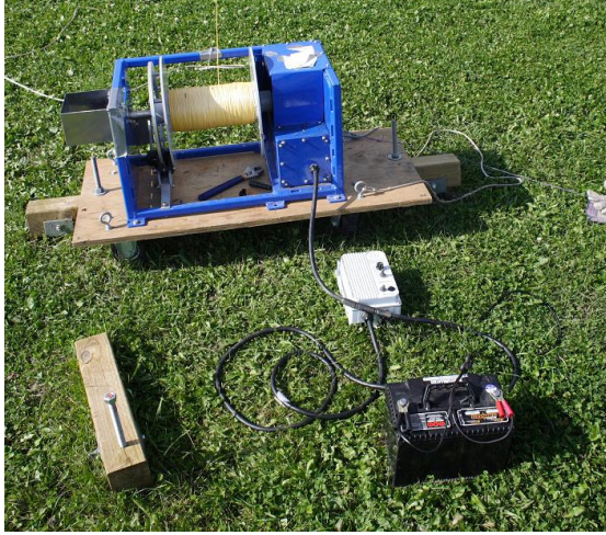
Figure 2.11 - CSW-1 winch with control box and battery power
