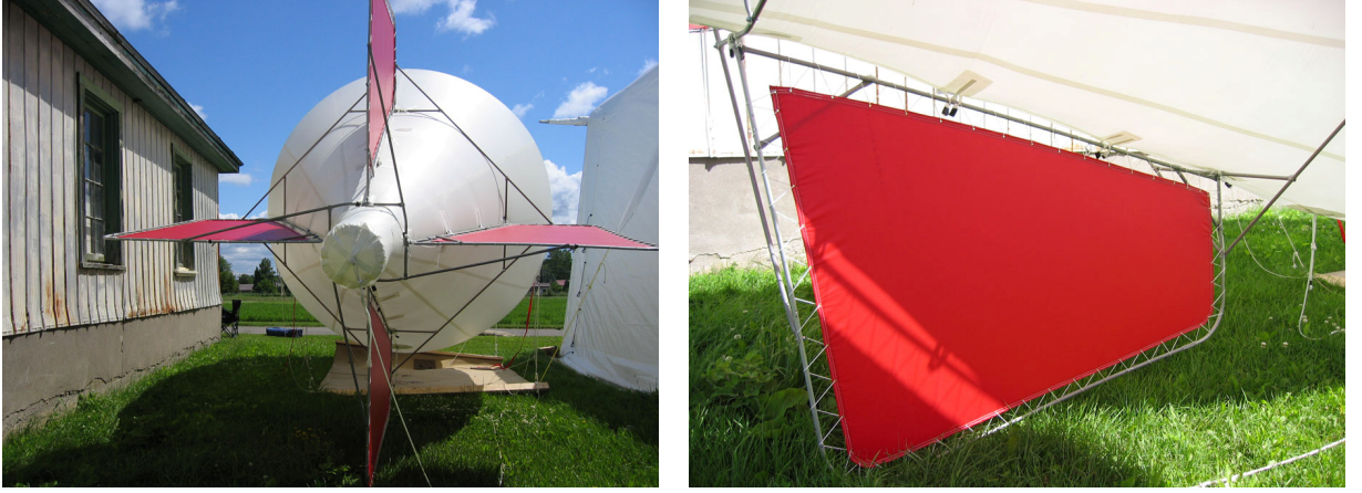
Figure 2.4 - Rear and side views of the TRF-900 aerostat showing the tail fin construction
