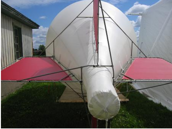
Figure 4.13 - Rear section of the TRF aerostat showing fin construction. Note that the control surfaces have not been installed.
