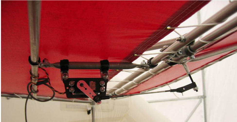
Figure 2.6 - Servo mounted on the fin with a pushrod
