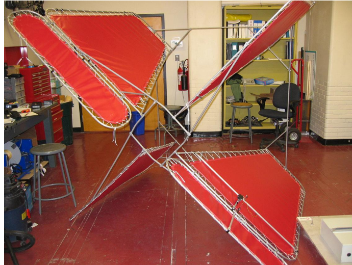
Figure 4.7 - Assembled tail section in the lab for measurements
