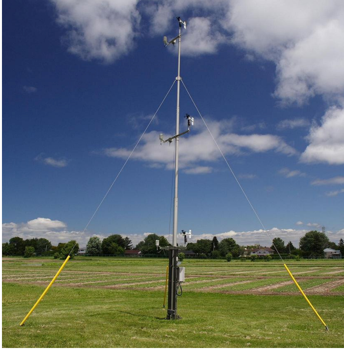
Figure 2.13 - Wind sensor tower with three Young sensors mounted at different heights
