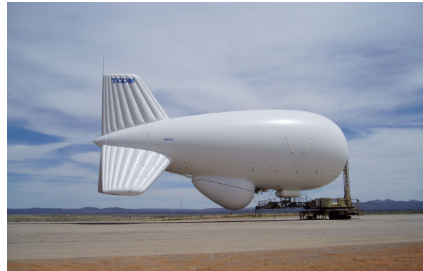
Figure 1.2 - TCOM's 17M aerostat with sensor package mounted to the belly [6]. This aerostat is commonly used for military applications.
