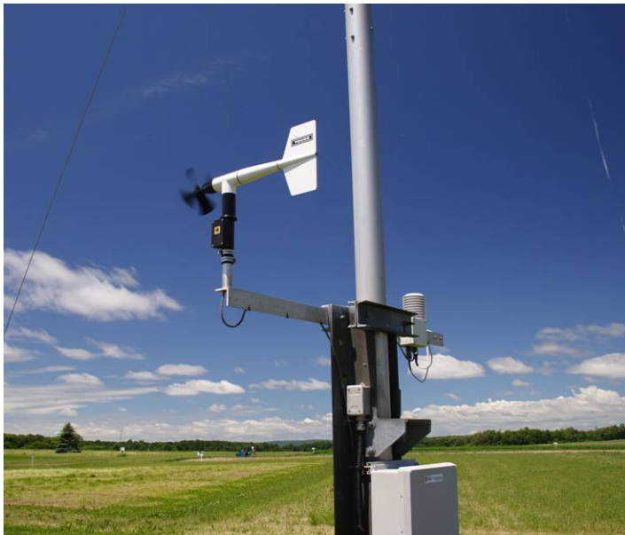
Figure 2.2 - One of three wind sensors mounted near the ground station
