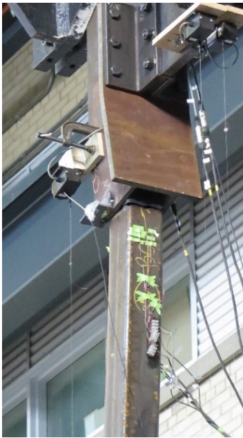
Figure 5.12: Tension fracture in Specimen 2 (1 st 2.0% EDR cycle)
