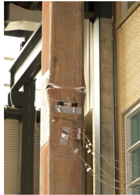
Figure 5.14: Low-cycle fatigue fracture in Specimen 5 (1 st 2.75% EDR cycle)
