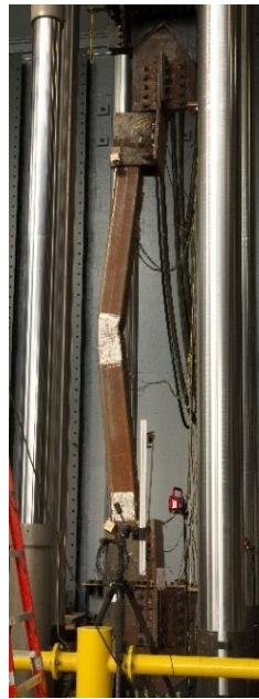
Figure 5.13: Onset of local buckling in Specimen 5 (1 st 2.25% EDR cycle)
