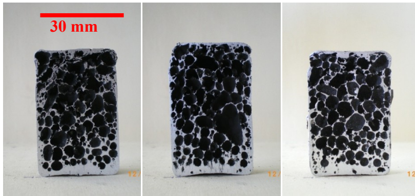
Al-3.5wt%Si-9.6wt%Zn foam Produced at 640 °C 1500 s
