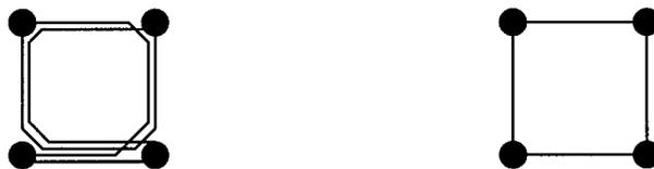
Figure 1.2: Bad (left) and good routing of a square with a good placement.
