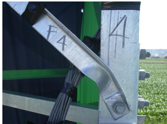
Figure 4.17 Failure of bracing members in Test 5
