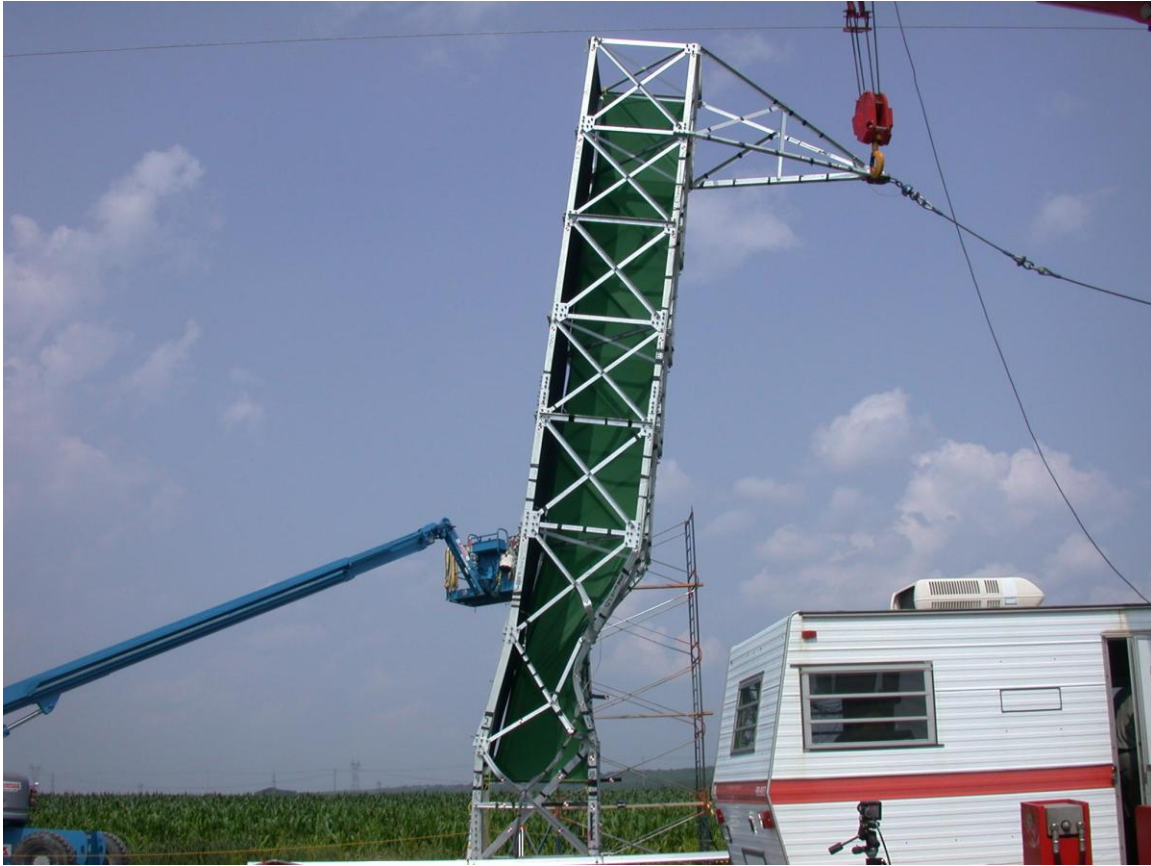
Figure 4.30 Deformed structure in dynamic bending (Test 12)
