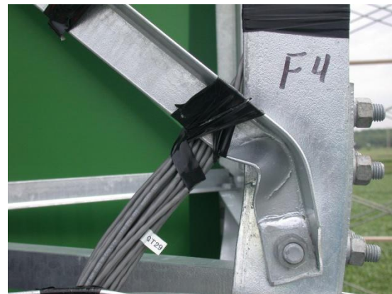
Figure 4.23 Failure of bracing members in Test 6
