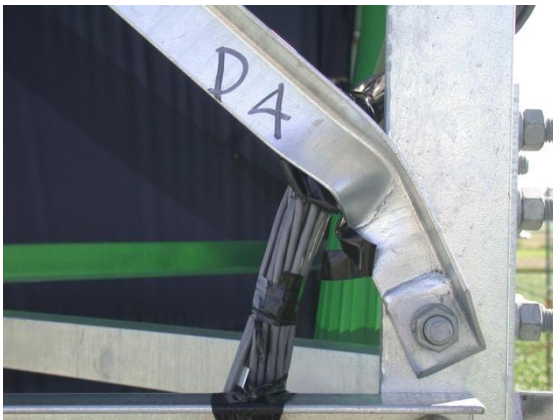
Figure 4.17 Failure of bracing members in Test 5
