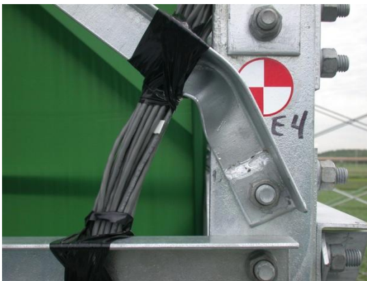
Figure 4.23 Failure of bracing members in Test 6
