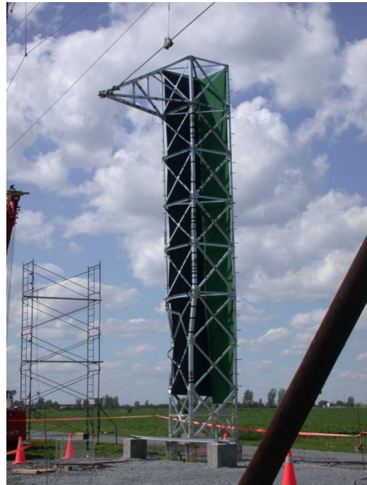
Figure 4.15 Deformed structure in pushover static torsion (Test 5)
