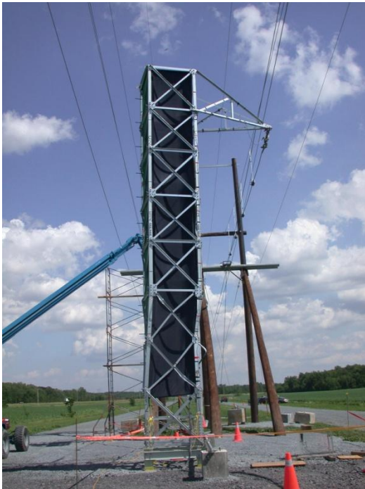
Figure 4.15 Deformed structure in pushover static torsion (Test 5)
