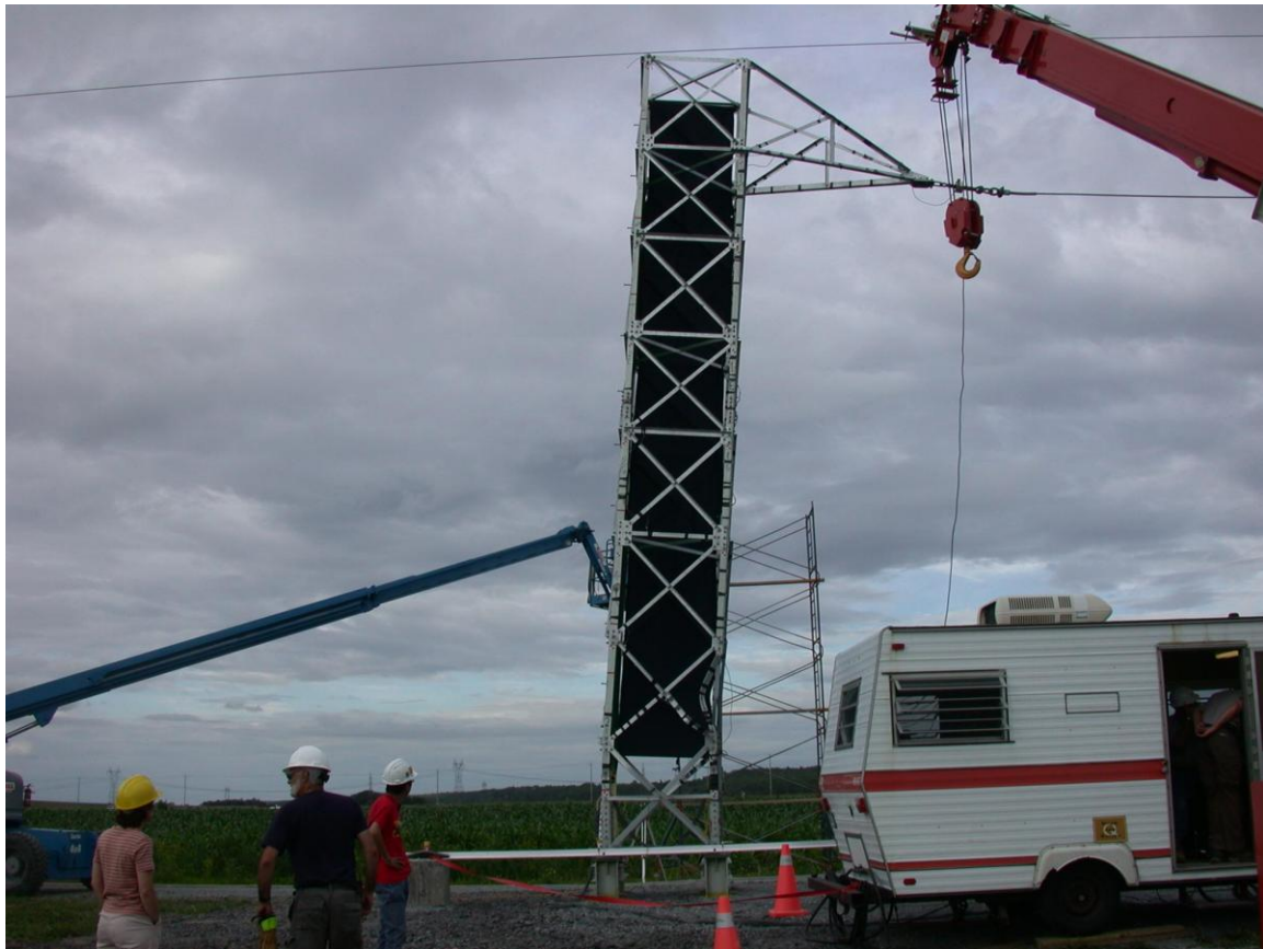
Figure 4.26 Deformed structure in static pushover bending (Test 11)
