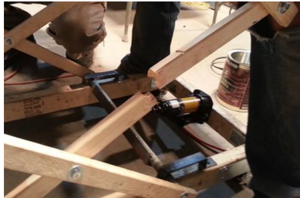
Figure 8: Failure of the wood in the initial prototype scissor lift.
