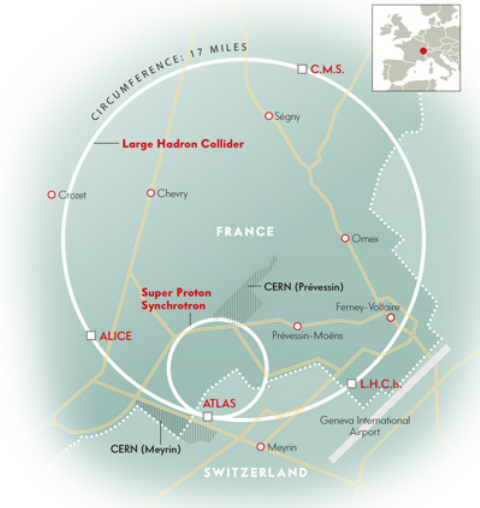
Figure 2.4: Map of the LHC’s geographical position with the four main detectors situated on the LHC ring [35]
