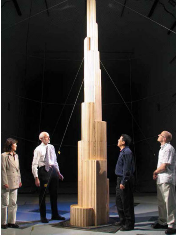
Figure 36: 1:50 scale model of top of Burj Khalifa in NRC's 9m x 9m wind tunnel
