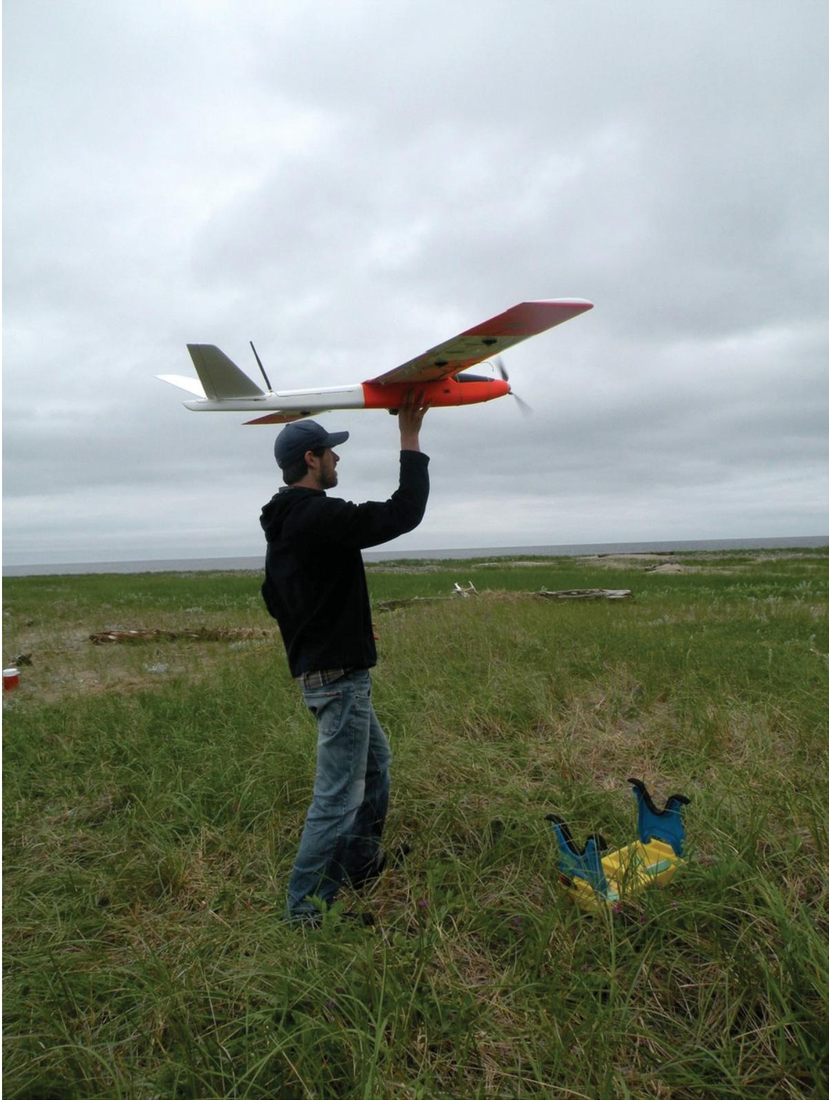
**Figure 3.** The hand-launched AI-multi electric unmanned aircraft prior to takeoff from the South Kouchibouguac Dune, Kouchibouguac National Park, New Brunswick, 2012.
