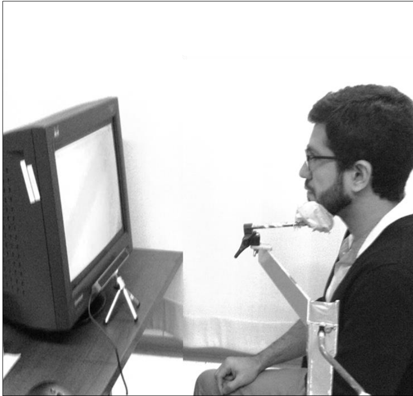
Figure 4.1 Psychophysical testing setup includes a computer monitor, chin rest, and eye tracker.
