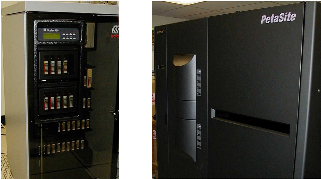
Figure 3.5 Tape library for long-term storage: a) ADIC Scalar 458; b) Sony PetaSite DMS 8800.
