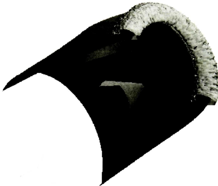
Figure 6.24: 3D ice accretion on the Boeing 737-300 inlet, rime ice accretion for 15° AoA and an inlet mass flow of 10.4 kg/s.
