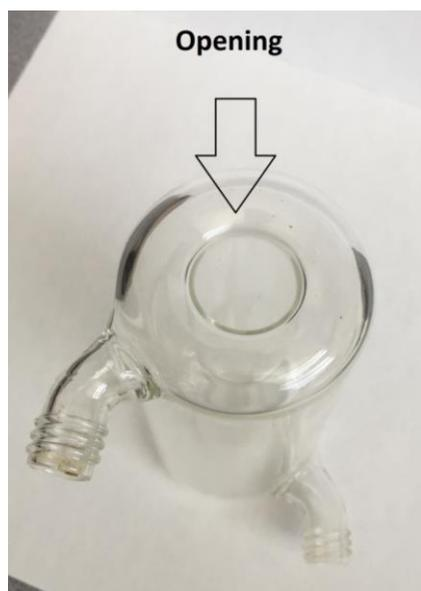
Fig. 3-5 View of the jacketed glass reactor from the top. The opening, where the liquid sample is inserted, is sealed by a top lid (not shown in this picture).
