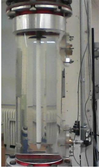
**Fig. 2.2.** Cantilevered cylinder enclosed in a transparent plexiglas test-section.
