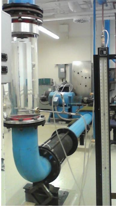
**Fig. 2.10.** Pitot-static tube and mercury manometer set-up for flow velocity calibration.
