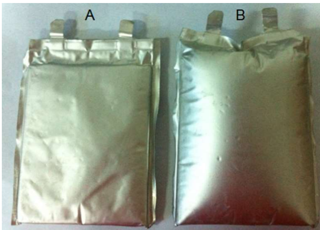
Figure 2.10. Images of LTO batteries after 1000 cycles, operated at (a) 25 °C and (b) 55 °C, respectively. The figures are modified from Figure 1 & 3 in Reference 2.74.
