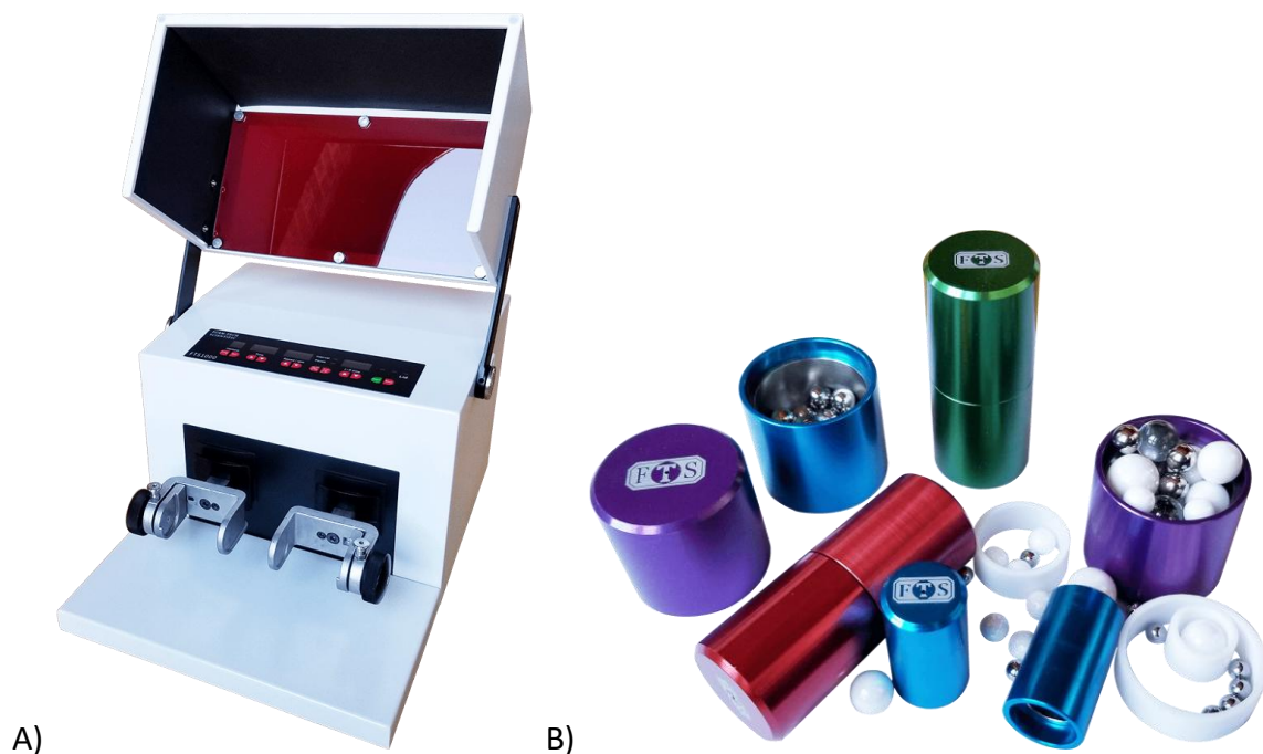
Figure 1.8: Equipment often used in mechanochemistry and mechanoenzymology. A) Standard benchtop shaker and B) typical milling jars and balls in a variety of sizes (images from: https://formtechscientific.com/ )
