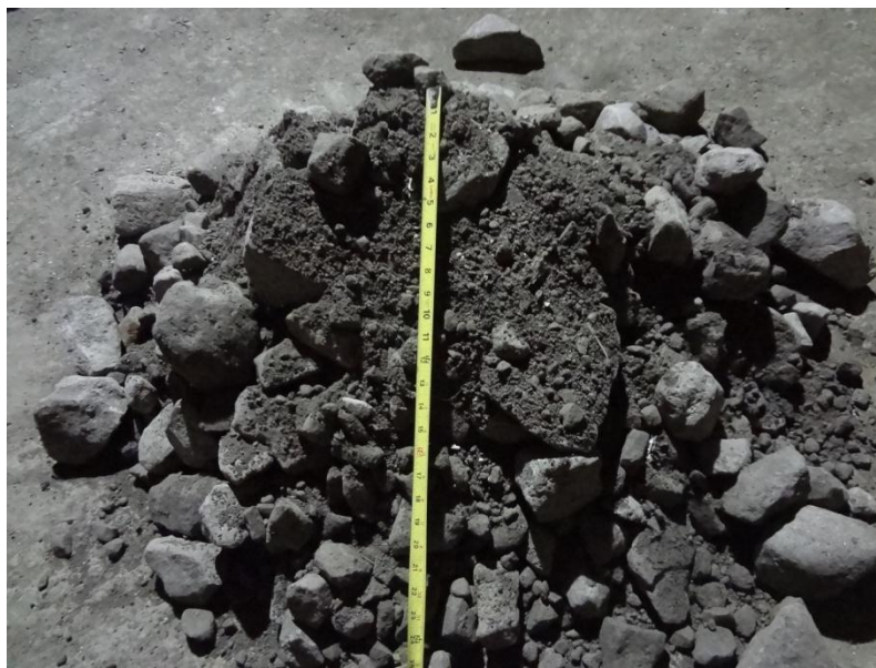
Figure 11: 600lb 5" Talbot curve graded aggregate pile for specimen 6a
