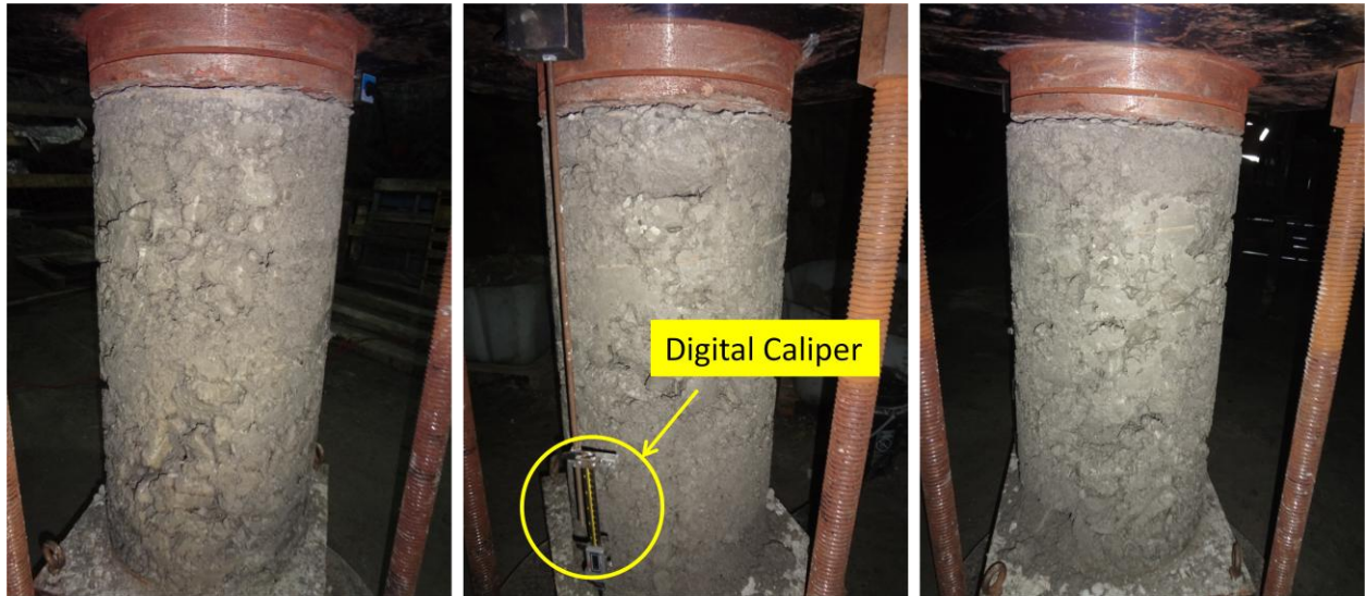
Figure 13: Specimen ready for testing. Digital caliper is placed between reaction plate and specimen base plate.
