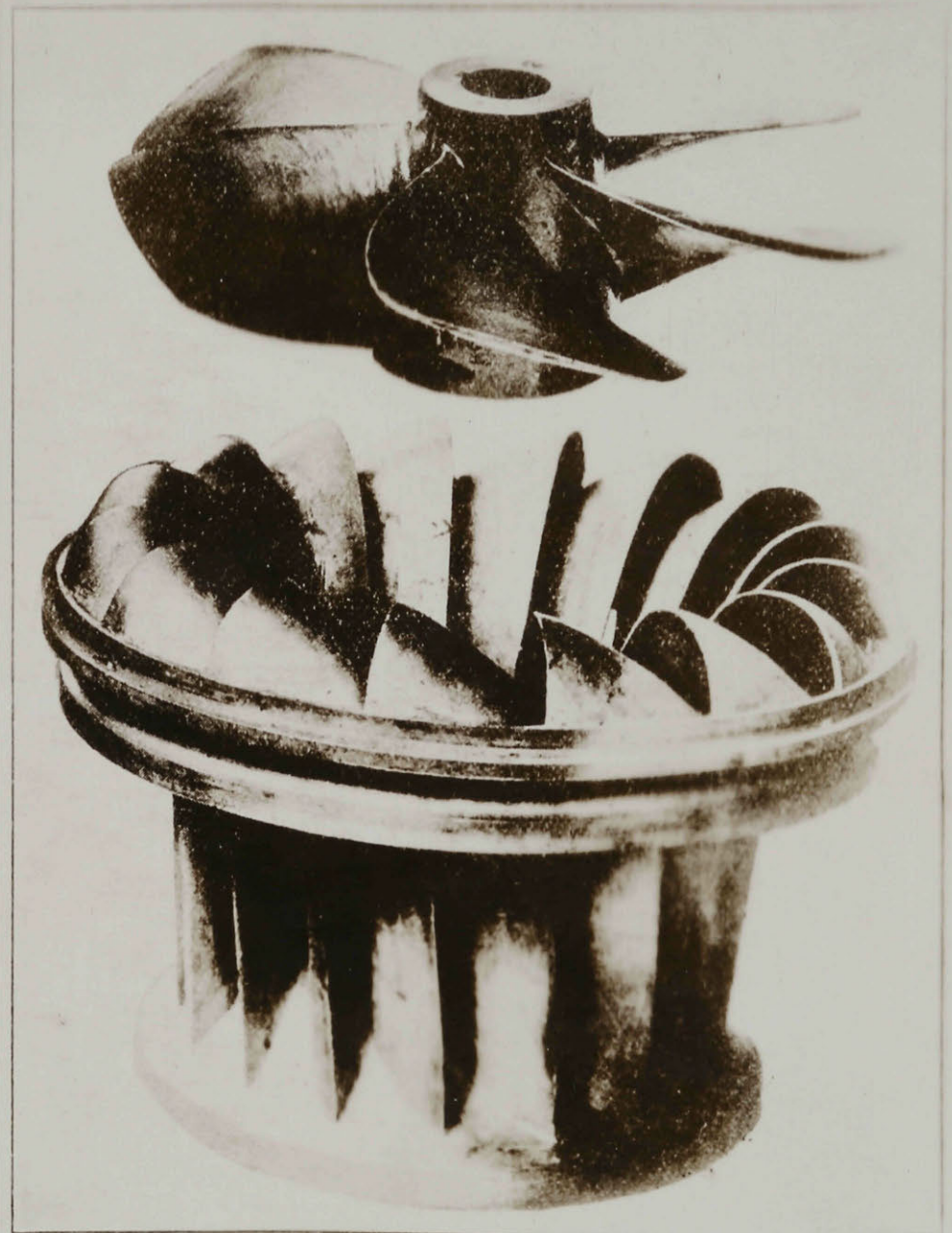
FIG. 50 Comparison between Propeller and Francis Types of Turbine Runners.
