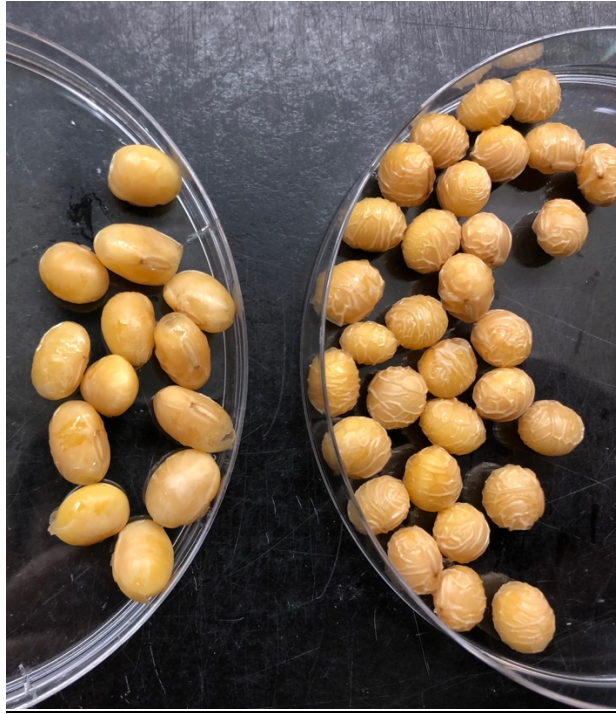
Figure 3.15 On left fissured seeds and on right non-fissured seeds after sodium hypochlorite test
