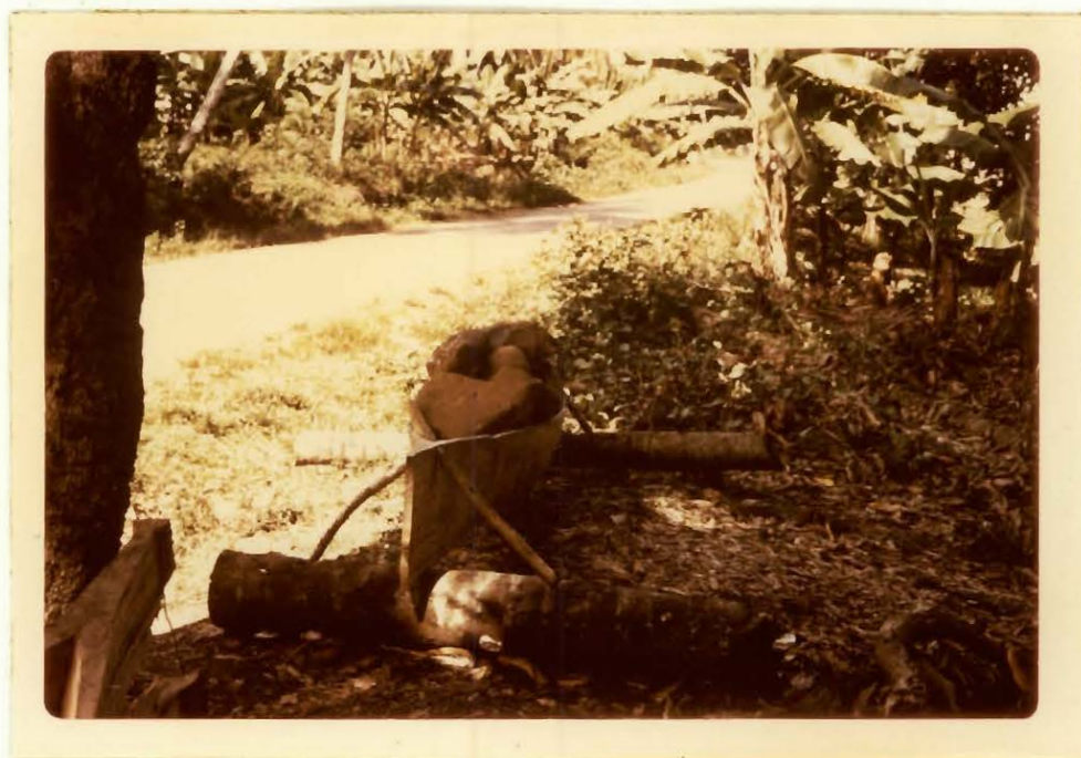
4 - Stretching the Hull. The second stage in building a traditional canoe.
