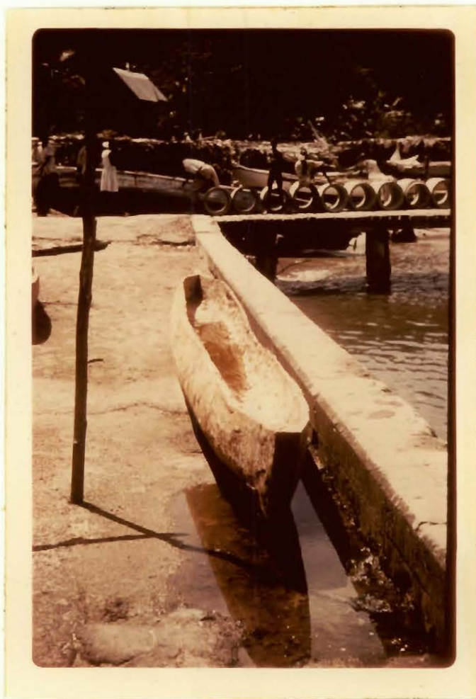
3 - Dug-out tree trunk. The first stage in building a traditional canoe.
