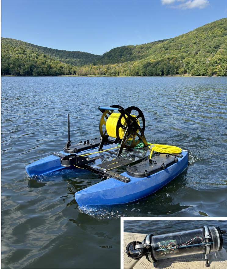
Figure 5.3: A picture of our robotic setup which includes the BlueBoat and the sensor unit.
