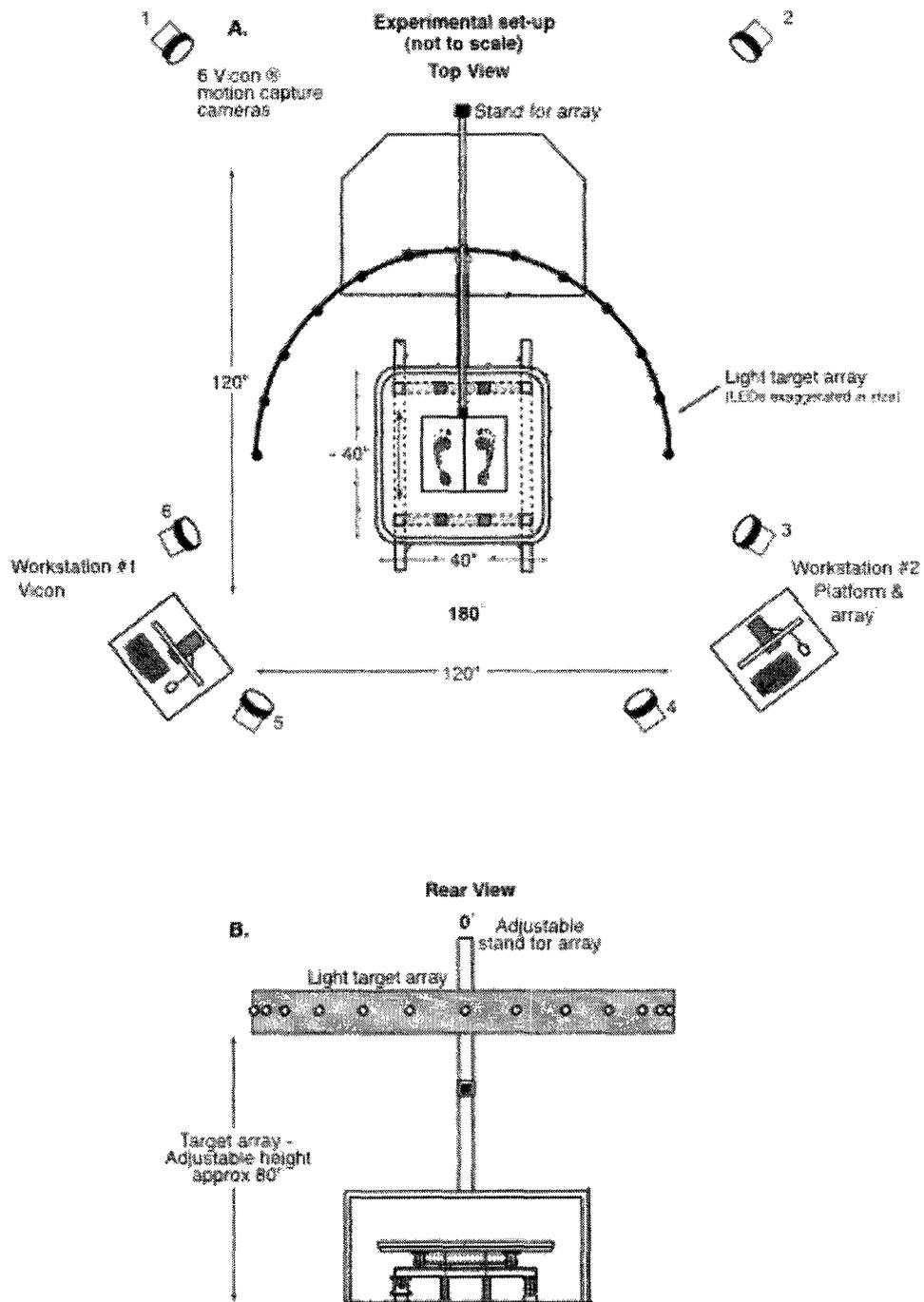
**Figure 3: (A) Top view of experimental setup (180° array of LED's in clockwise direction from left to right); (B) Rear view of light target array and platform (Reproduced with kind permission from P. Stapley).**
