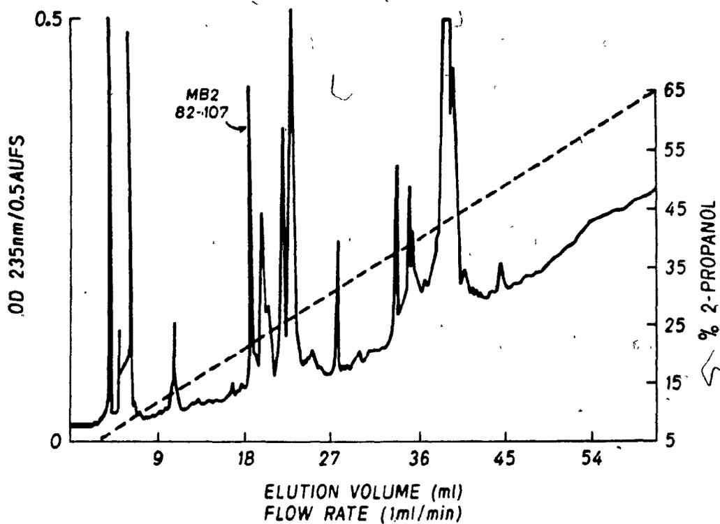
Figure 31. Chromatographic profile on HPLC u-Bondapak C-18 analytical column of undialysed flow through material from CMC of pig pars distalis extract.
