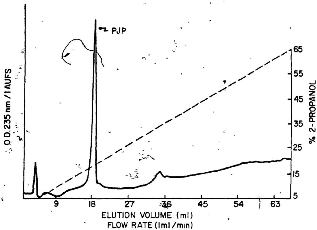
Figure 32. Chromatographic profile on HPLC u-Bondapak C-18 analytical column of the final purification of the porcine joining peptide.
