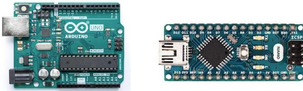
Figure 5-6. Image of Arduino UNO (left) and Arduino Nano (right)
