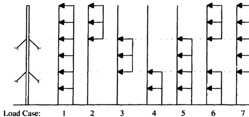
Figure 5-2. Wind load cases for patch load method. [37]
