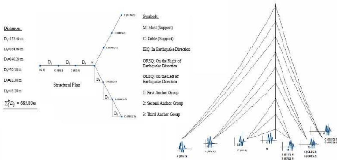
Figure 2-2. Schematic asynchronous ground motion input at support points for the 607 m mast [20].
