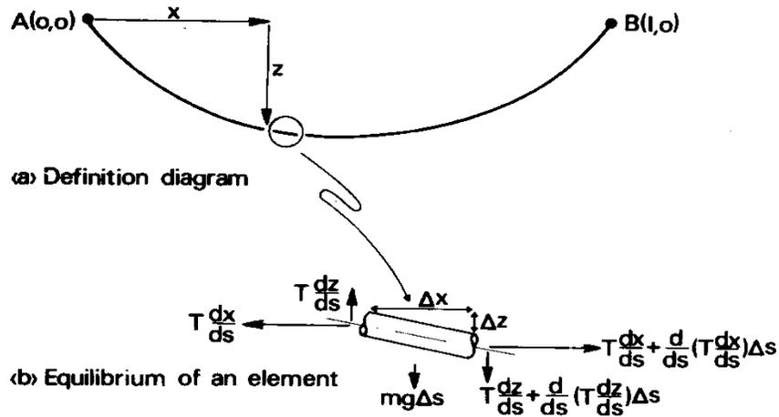
Figure 3-1. Illustration of the horizontal and the vertical equilibrium of an isolated element of the catenary. [29]
