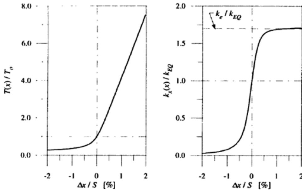
Figure 3-3. Example of static tension and horizontal stiffness curves for single guy [30].
