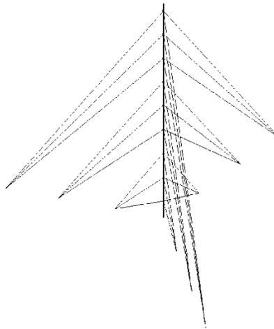
Figure 2-1. Geometry of the 607 m mast by Faridafshin (2006) [19].
