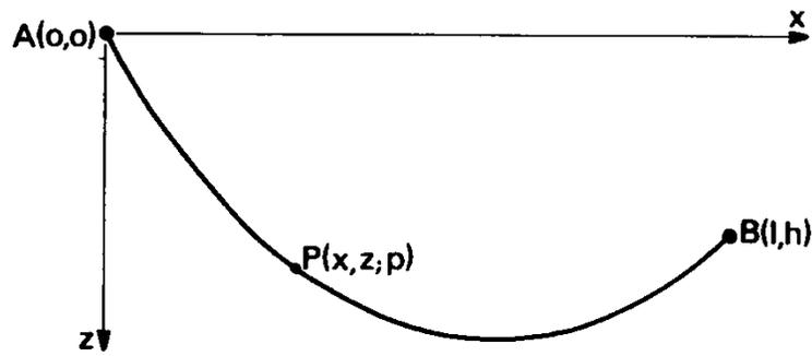
Figure 3-2. Coordinates for the elastic catenary. [29]
