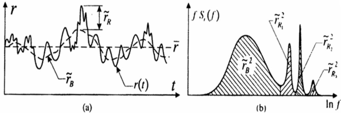
Figure 5-1. The response of a guyed mast to wind; (a) time history, (b) Power spectra. [37]
