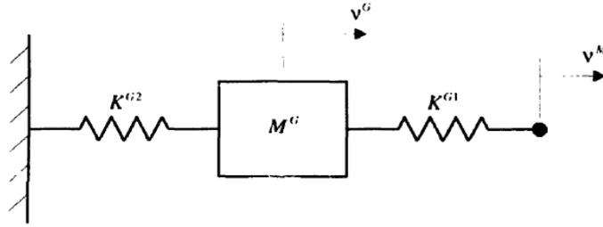
Figure 3-8. Equivalent spring-mass guy model.
