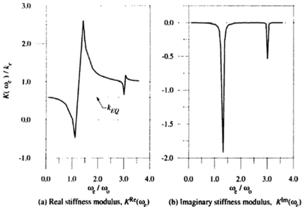
Figure 3-7. Complex guy stiffness vs. frequency [6].
