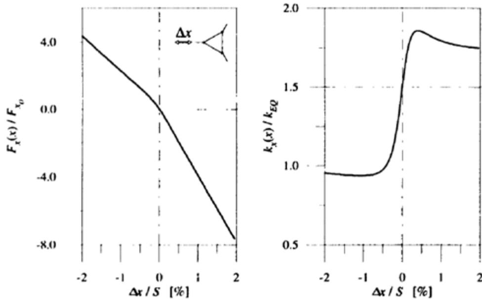
Figure 3-4. Example net horizontal reaction force and stiffness for a group of 3 guys [30].
