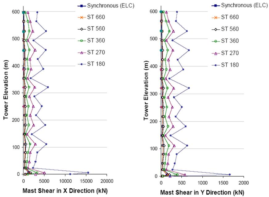
Figure 2-5. Envelope of the mast shear distribution in  $X$  and  $Y$  directions; EI Centro; 607 m mast. [19]
