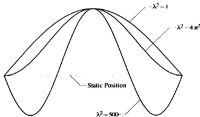
Figure 3-6. Variation in the first symmetric mode shape with  $\lambda^2$ . [6].
