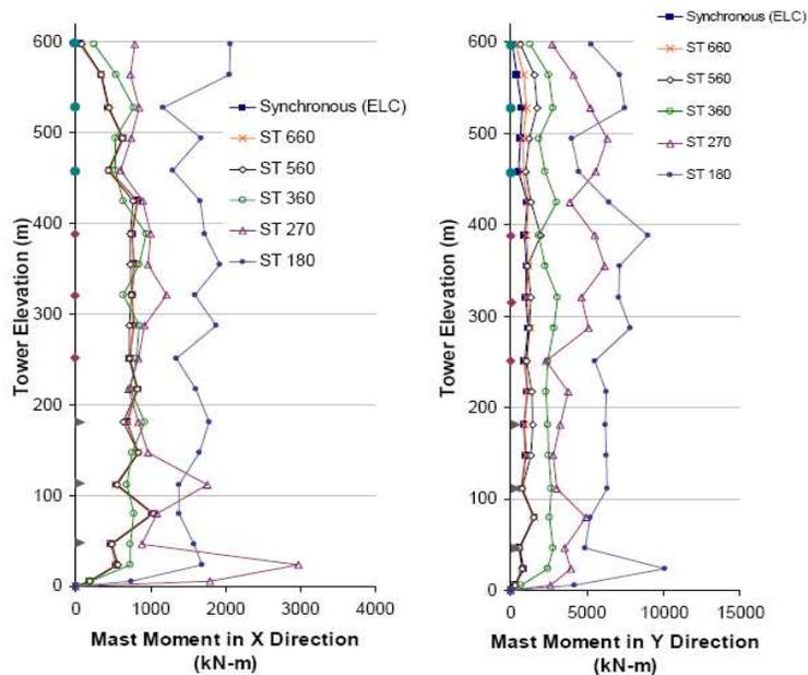
Figure 2-6. Envelope of the bending moment distribution in  $X$  and  $Y$  directions; EI Centro; 607 m mast. [19]
