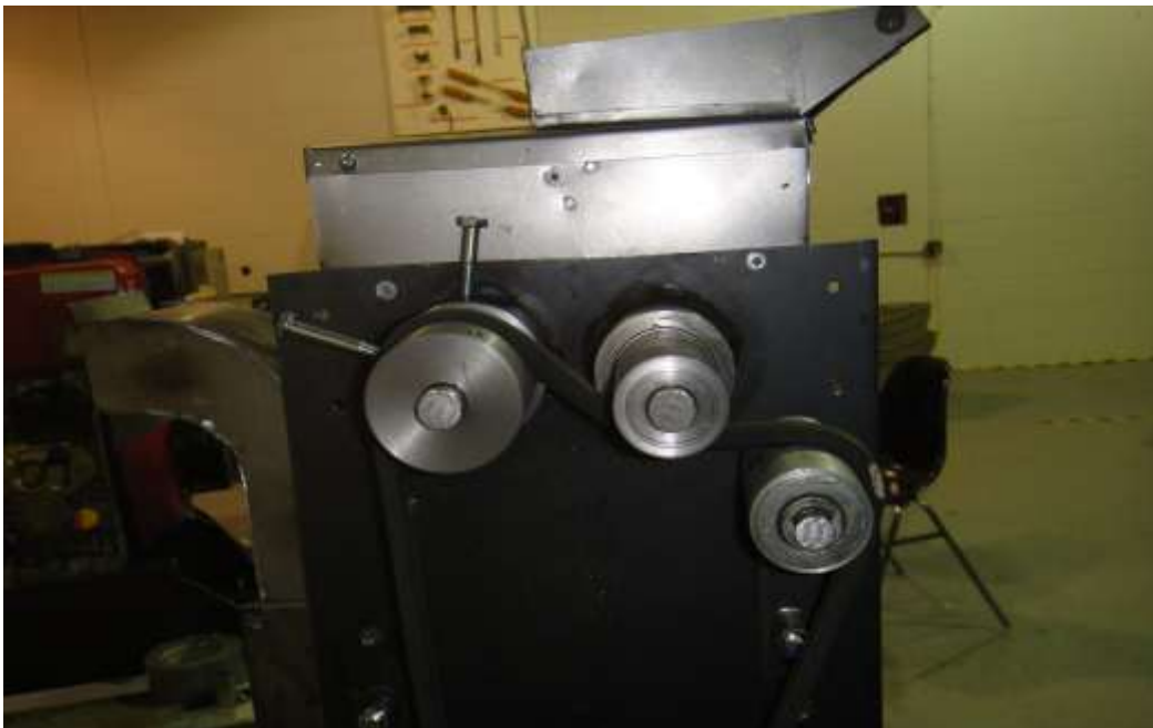
Figure 41 - Rubber Roller and Idler Pulleys
