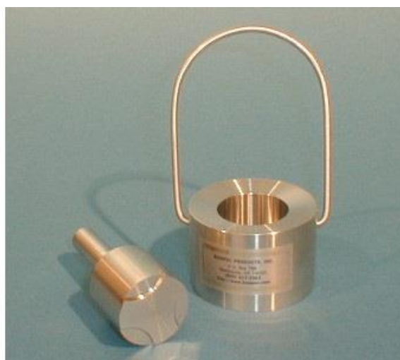
Figure 4.1 An image of a biopulverizer with a steel piston. Depicted from: https://www.labcompare.com/1258-Laboratory-Mill/12607956-BioPulverizer/
