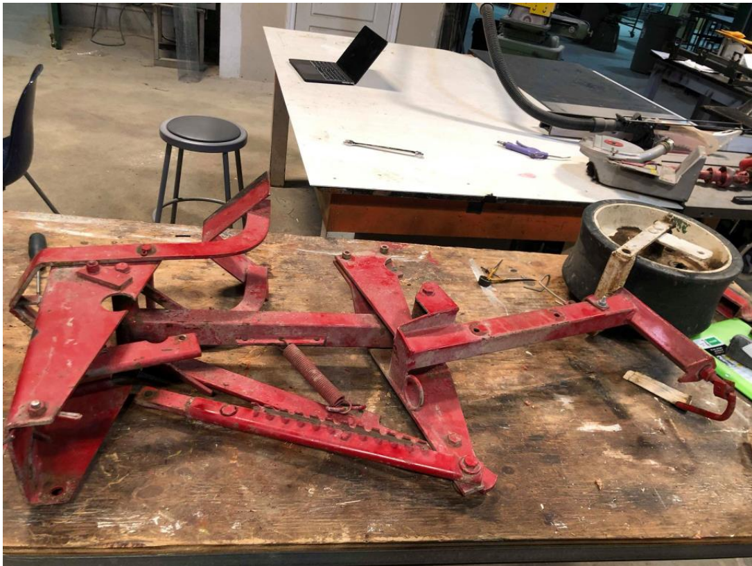
Figure 9. Disconnected vacuum seed metering device with power transmitting mechanism.
