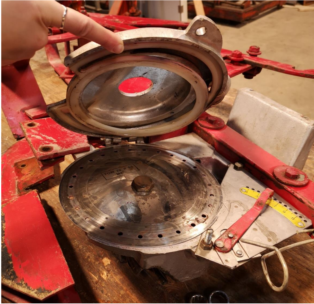
Figure 8. Metering plate inside of seed metering device onto which seeds sucked by the vacuum connected by tube underneath.
