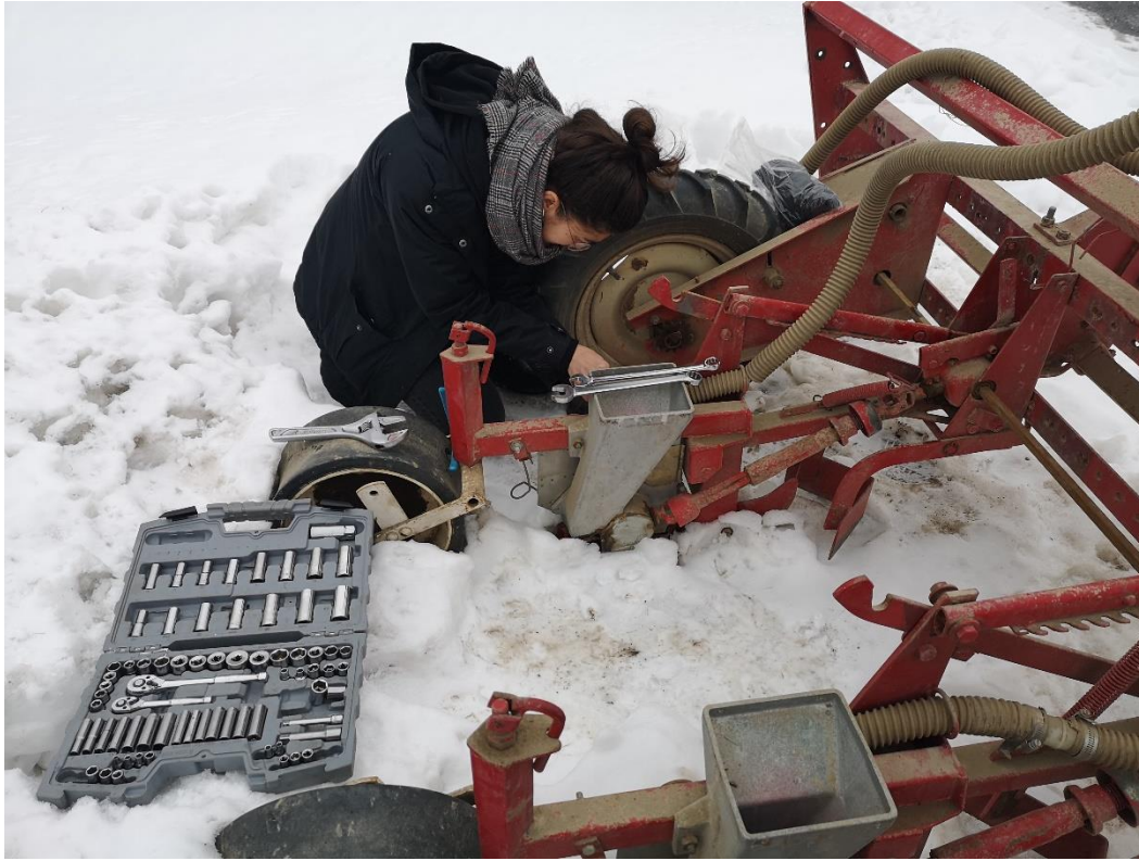
Figure 7. Team member, Leen, unbolting connections between seeder and single row unit.
