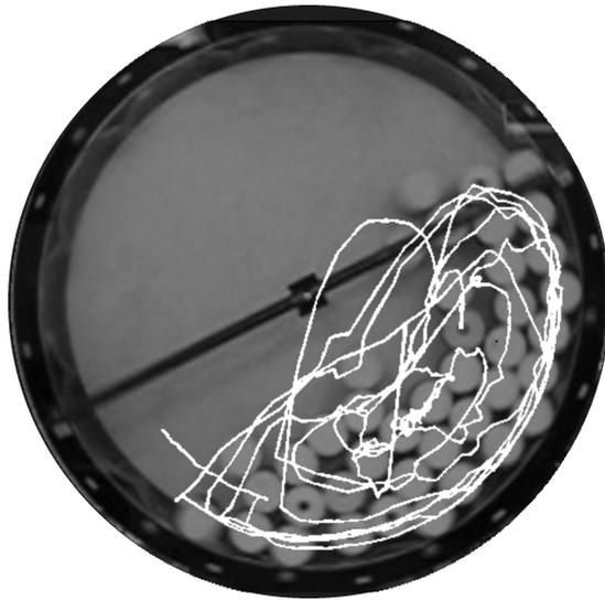
Figure 4–4: A picture of the operating mill with a measured instrumented ball trajectory overlay
