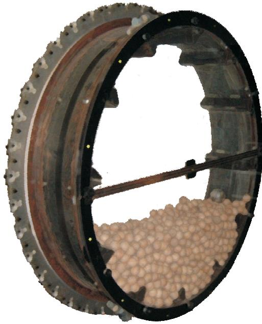
Figure 3-5: The laboratory mill
