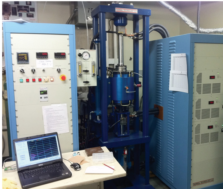
Figure 3.3: The Thermal Technologies SPS used for powder consolidation.
