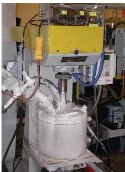
Figure 3.2: The Union Process mill used for grain refinement of the NiCoCrAlY powder.
