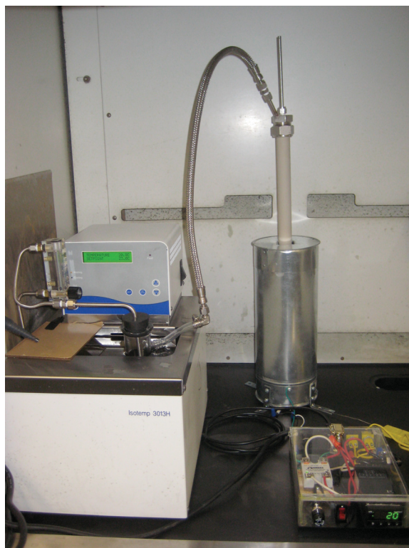
Figure 3.8: Apparatus for controlled-environment static oxidation tests.
