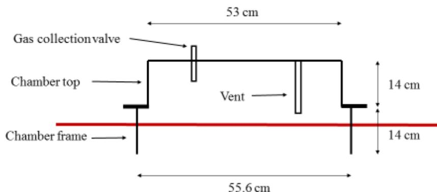
Figure 3.7: Static chamber design.
