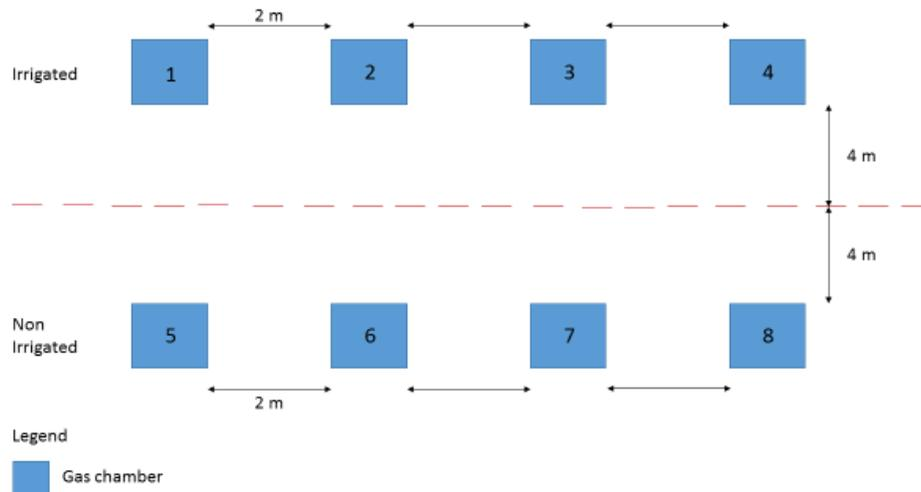
Figure 3.4: Diagram of the GHG sampling layout.
