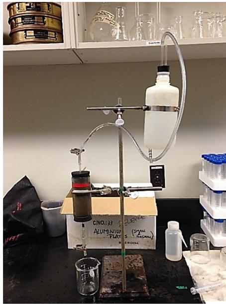
Figure 3.9: Saturated hydraulic conductivity set up in lab (Lloyd, 2015).
