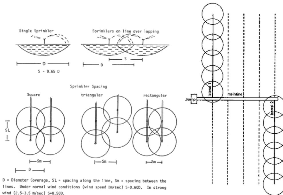
Figure 2.2: Hand moved over head sprinkler system (left) and profile of wetted soil under sprinklers (right) (Brouwer et al. (1985); Phocaides (2000)).
