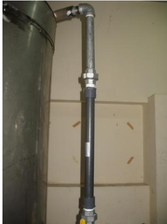
Figure 12 – The static mixer connected to Reactor A
