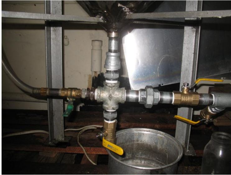
Figure 10 - The 4-way valve with the height-gage attachment
