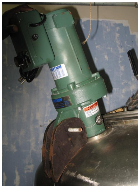
Figure 8 – The electric mixer with the mounting brackets
