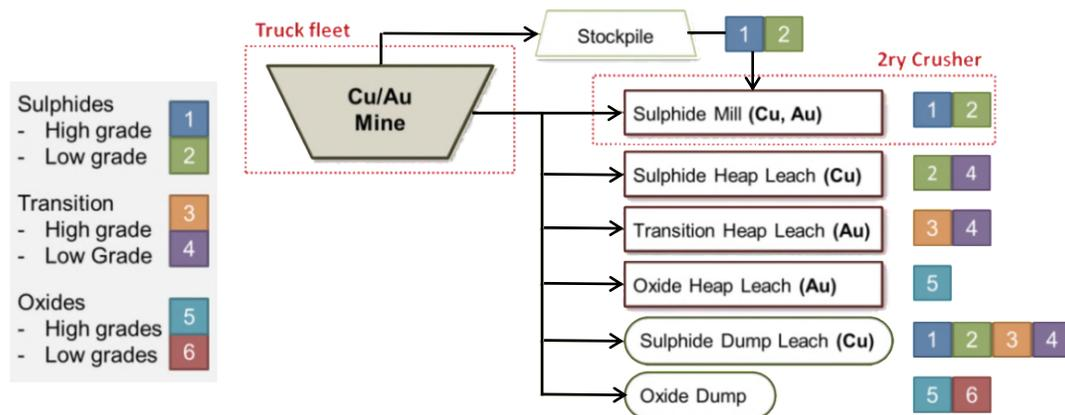
Figure 5-2 Mining complex layout with material allowed and metal produced per destination
