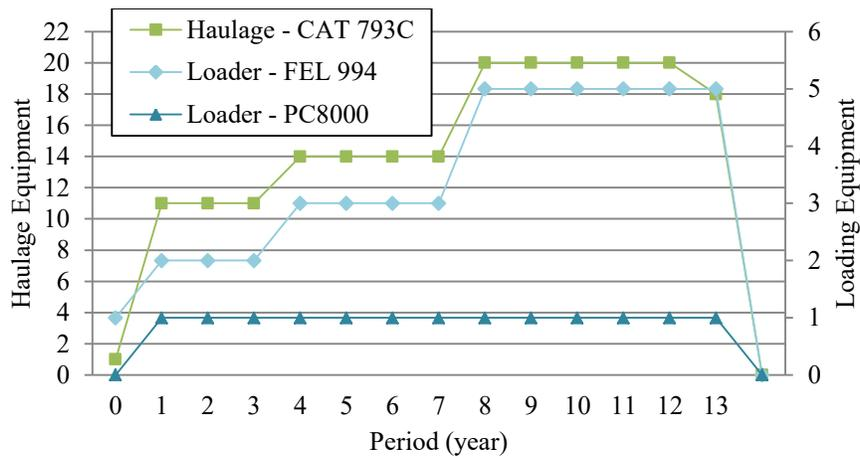
Figure 2-6 Equipment type and model acquisition schedule per period
