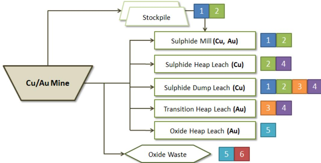
Figure 3-4 Diagram of processing streams available and the material types accepted
