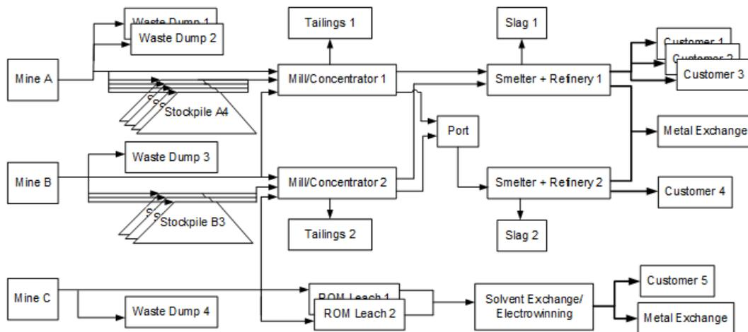
Figure 1-1 Diagram of a mining complex (Goodfellow, 2014)
