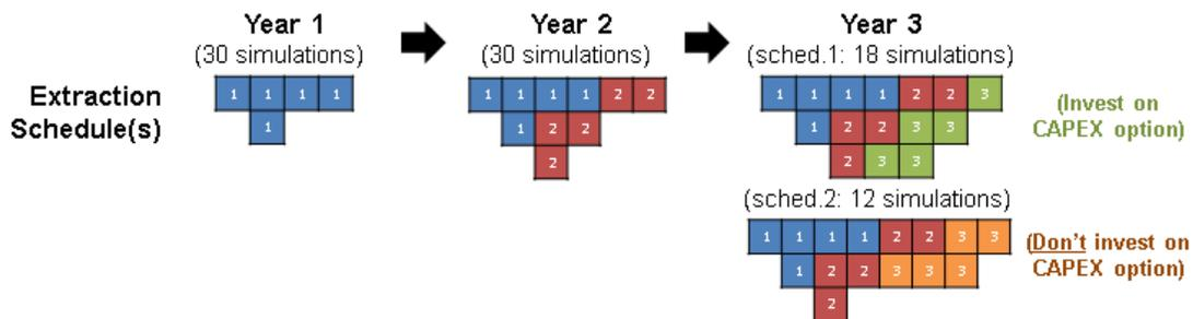
Figure 4-1 Example of including investment alternatives in the optimization process
