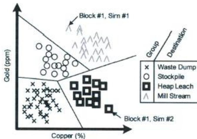
Figure 3-1 Creation of 4 clusters according to gold and copper concentration.
