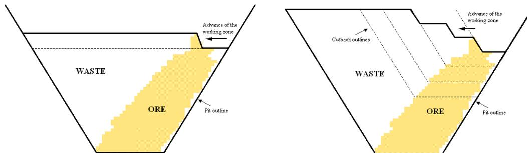
Figure 2-1 Schematic representation from (Whittle, 1999) of the (left) worst and (right) best case mining schedule.
