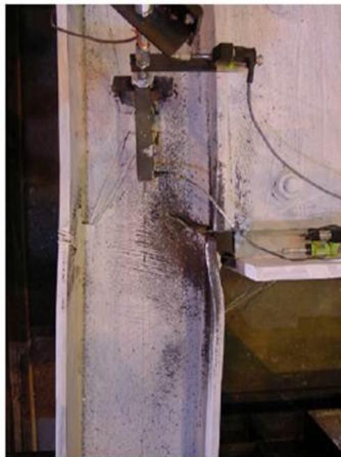
Figure 6.6 Ductile tearing of the north lower story column of the 2-story SCBF (Uriz, 2005)
