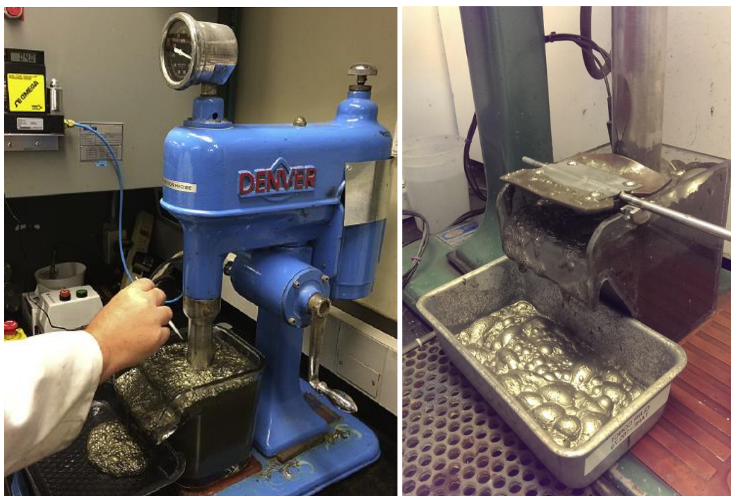
Figure 3.7 – (Left) Denver D12 laboratory flotation machine, reproduced from Wills and Finch (2016) [1] ; (right) cell equipped with automated froth paddle.
