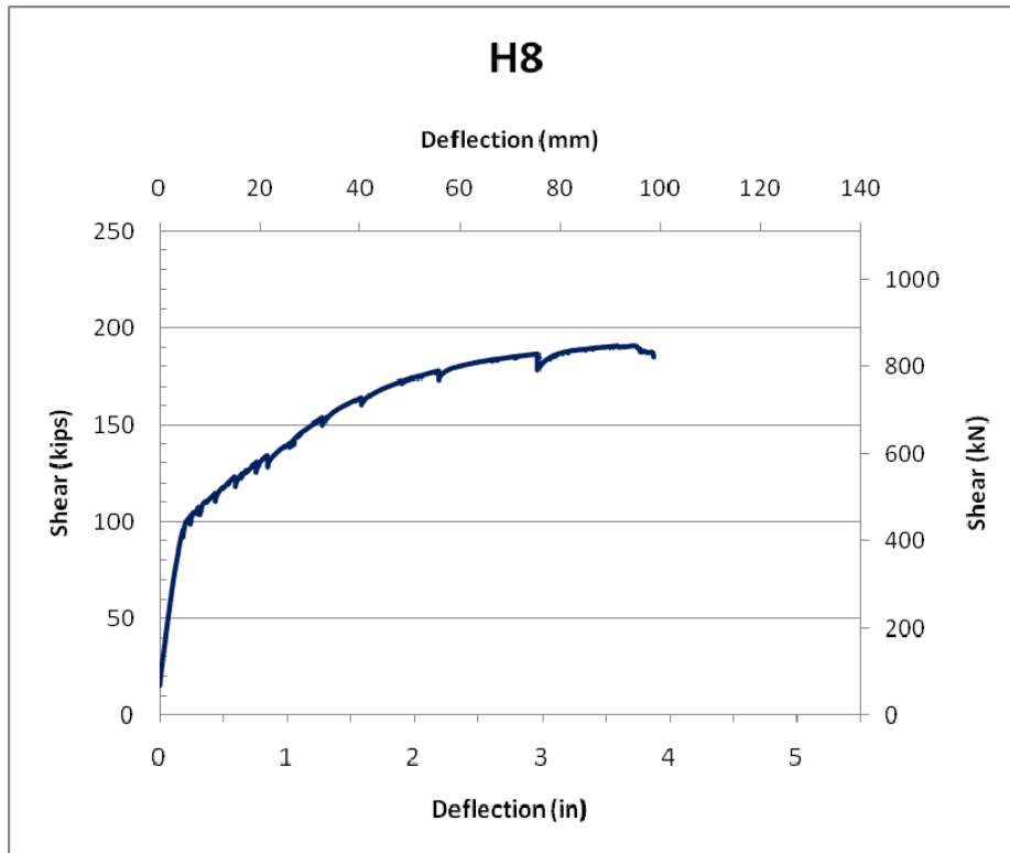
Figure 46: Shear versus deflection at load point – Specimen H8
