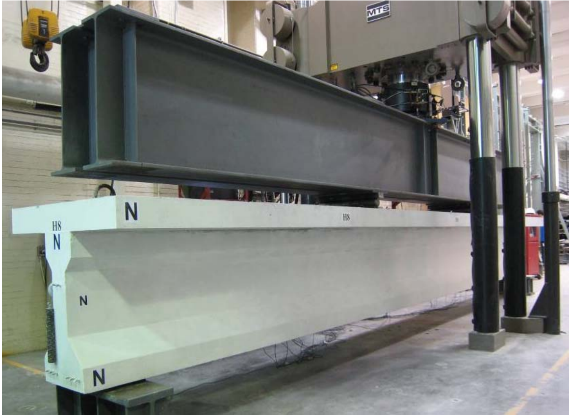
Figure 39: Specimen before testing
