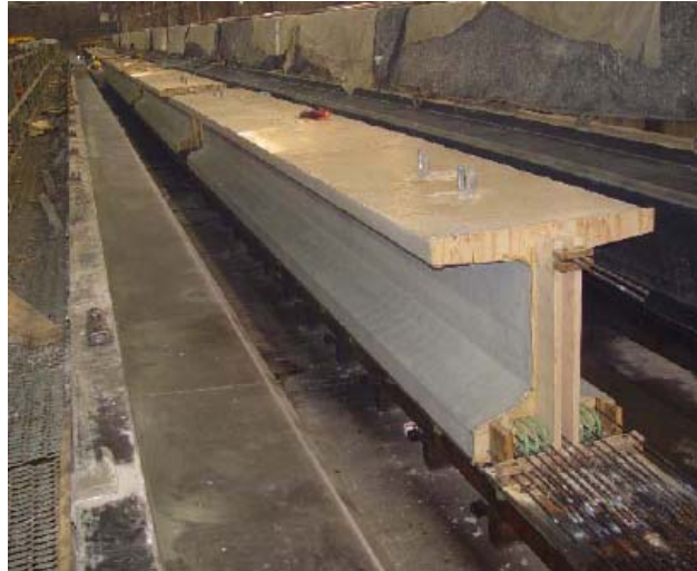
Figure 7: Flame cut unstressed strands at bulkhead (Naito, Brunn, Parent and Tate, 2005)
