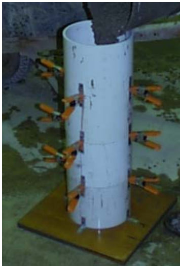
Figure 12: Column segregation test (National Ready Mixed Concrete Association, 2008)
