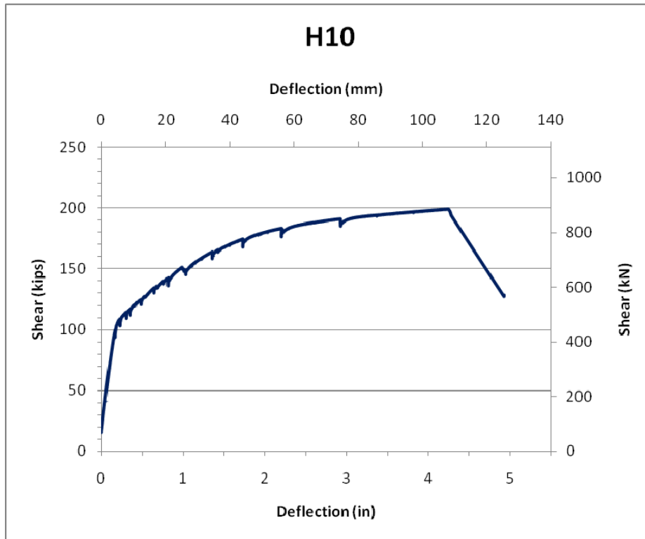
Figure 48: Shear versus deflection at load point – Specimen H10
