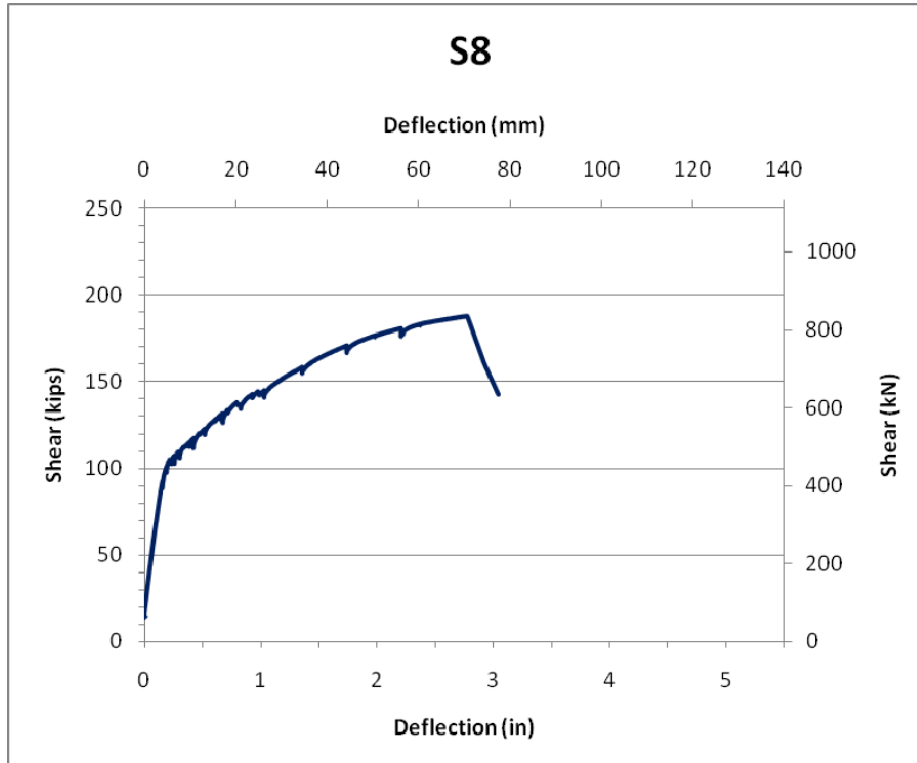
Figure 47: Shear versus deflection at load point – Specimen S8
