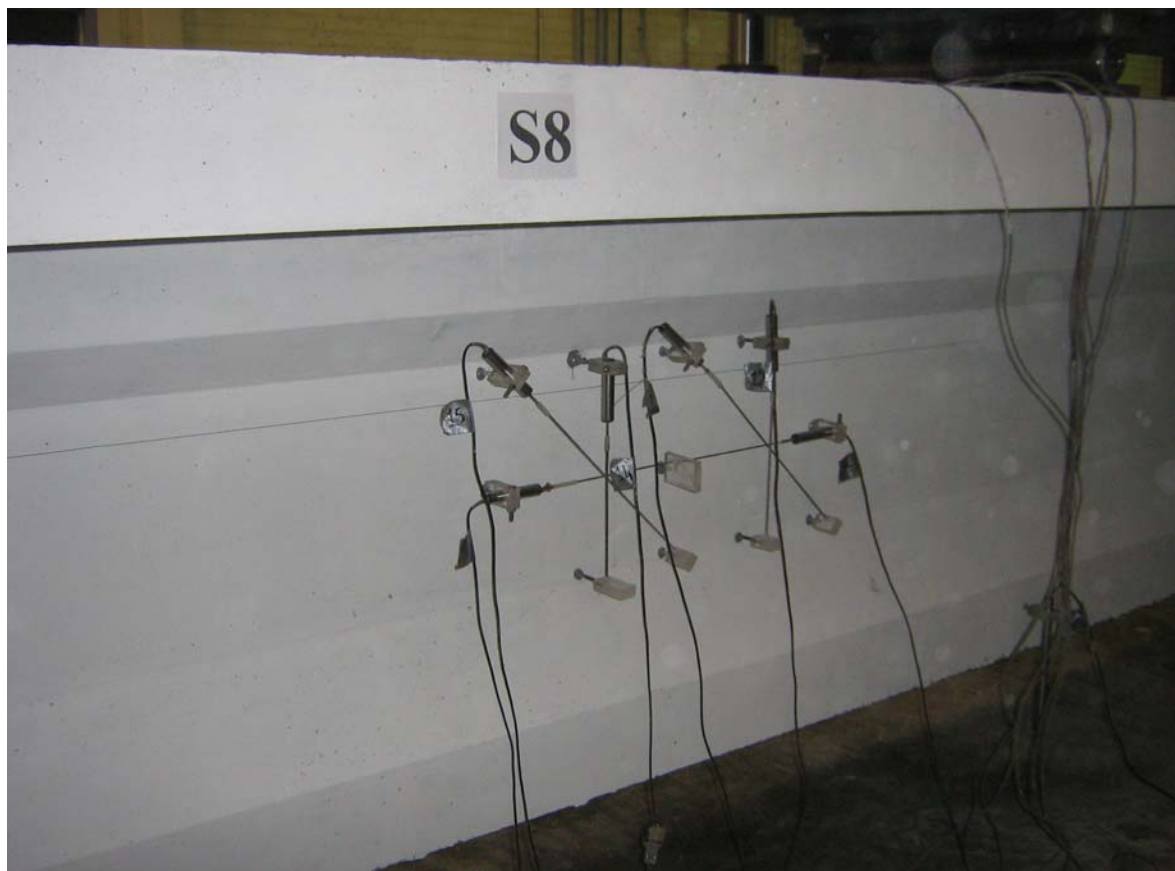
Figure 38: Test setup and locations of LVDTs
