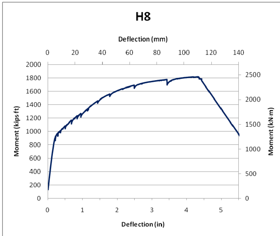
Figure 41: Moment versus central deflection – Specimen H8
