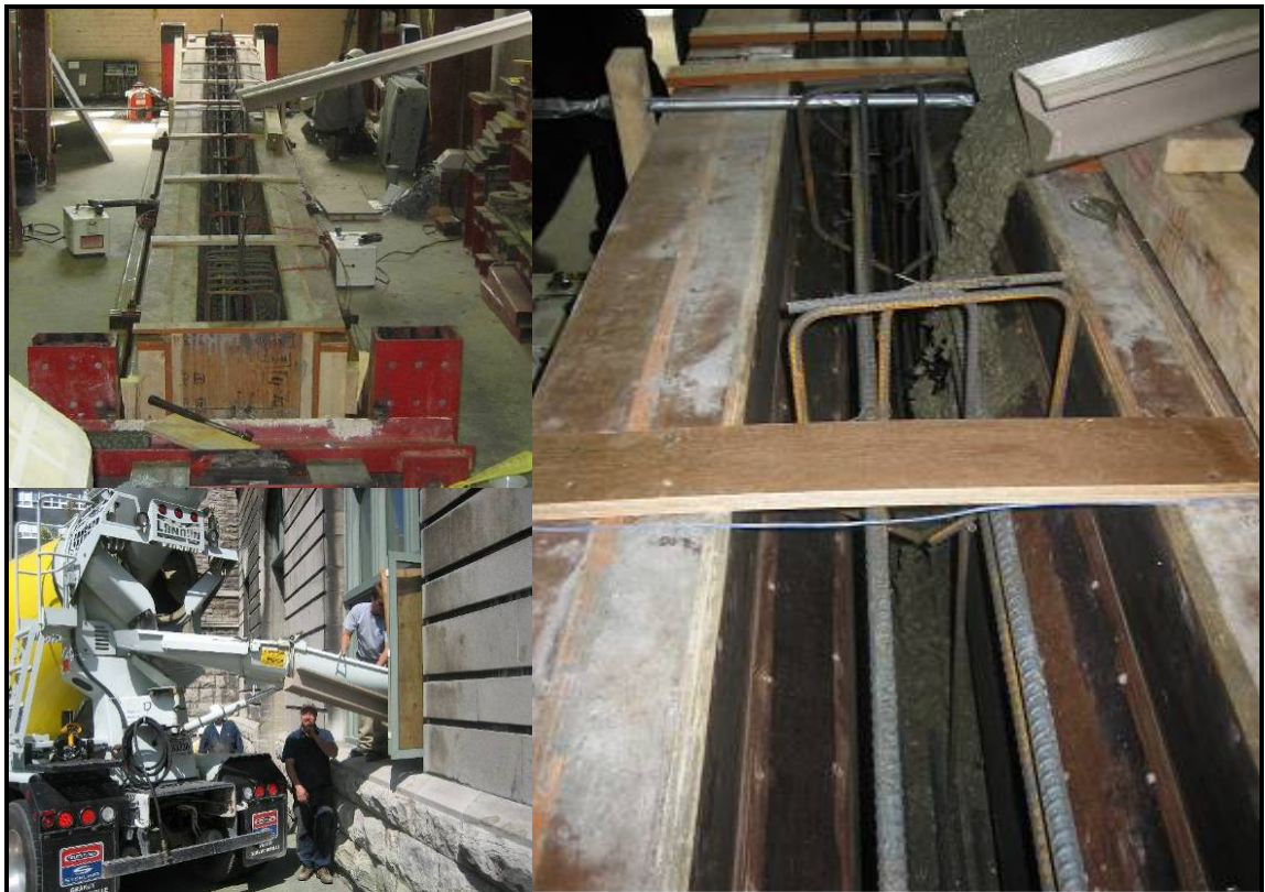
Figure 24: SCC girder casting operation (Khayat and Mitchell, 2009)
