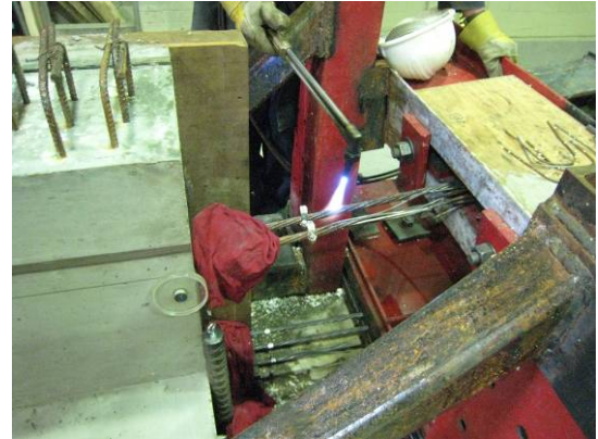
(b) Release of inclined strand
