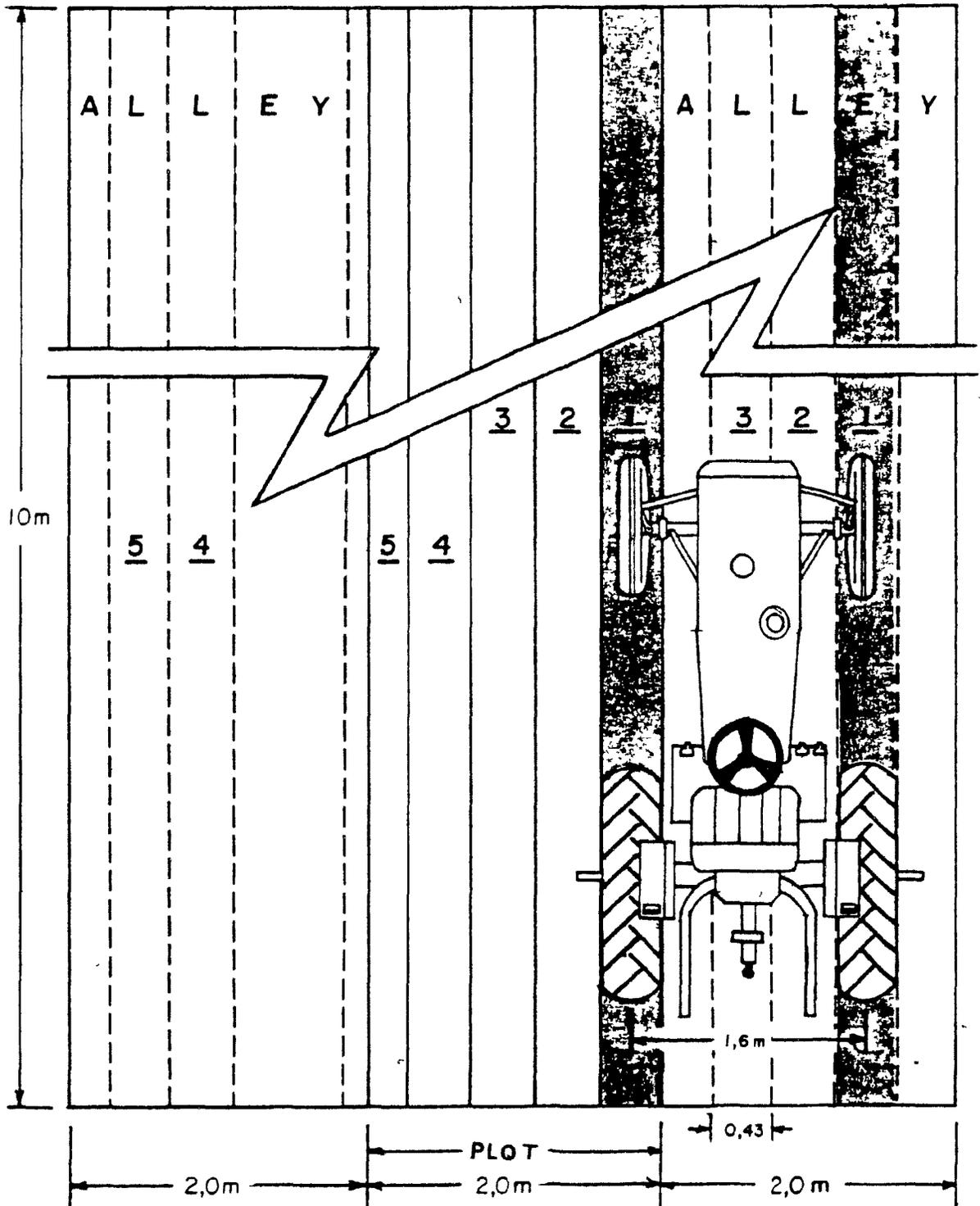
Figure 4.2 The path followed by MF-165D tractor for compacting the soil uniformly.
