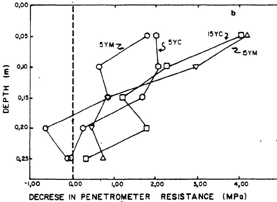
Figure 5.10 Observed changes in penetrometer resistance profiles due to tillage treatments.
