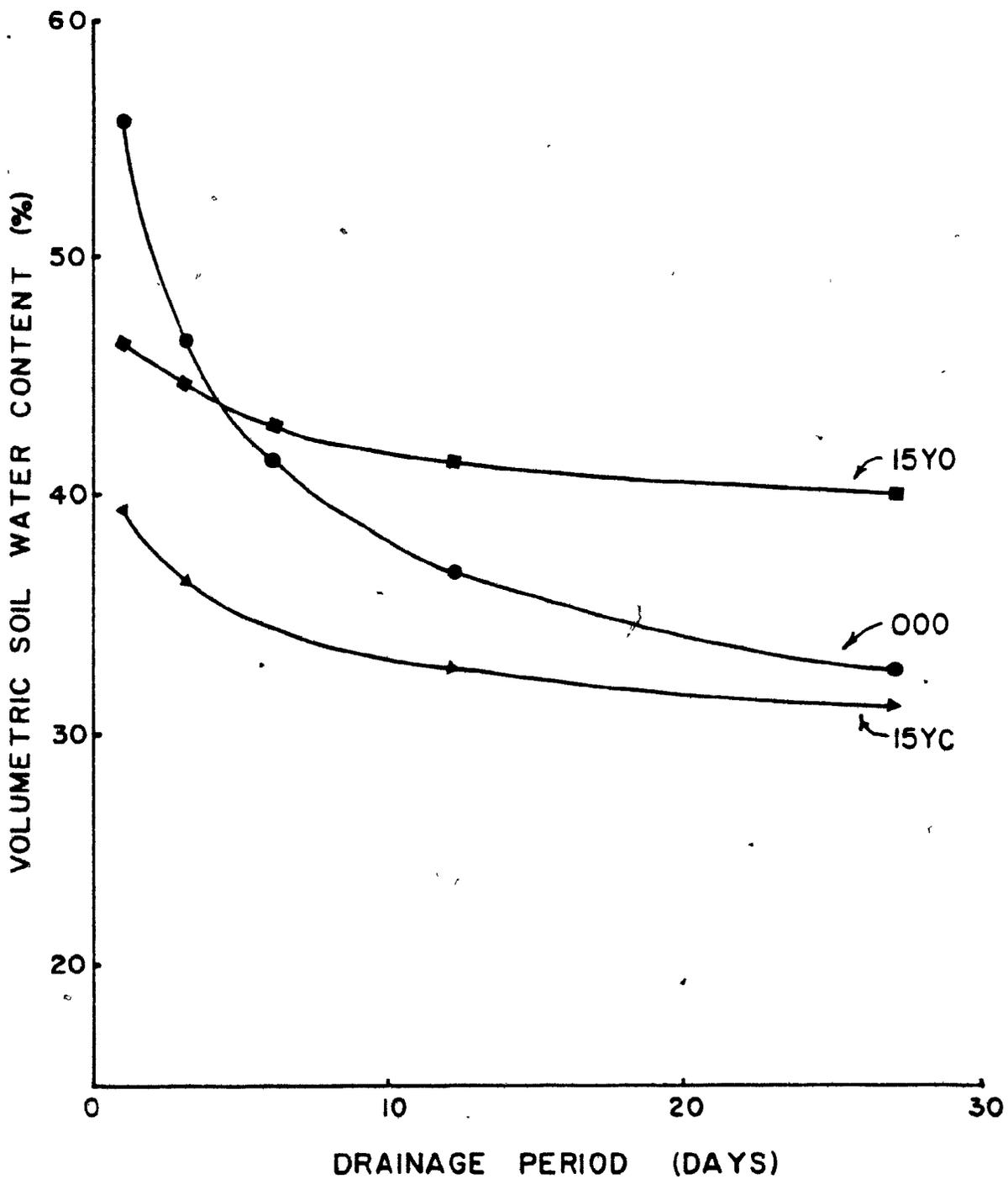
Figure 5.18 Volumetric moisture content versus drainage period at 0,25m depth.
