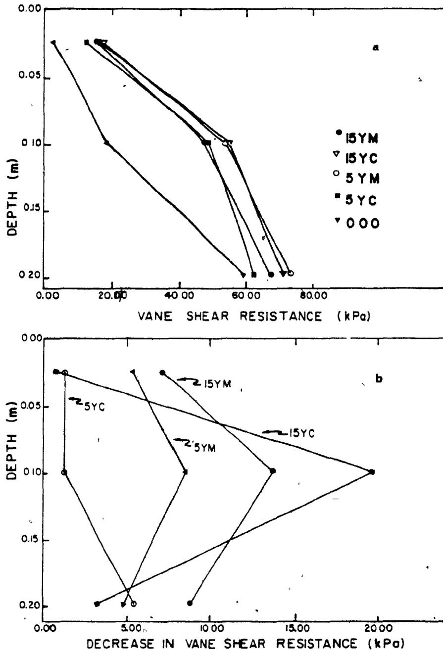
Figure 5.13 Observed changes in vane shear resistance profiles due to tillage treatments.
