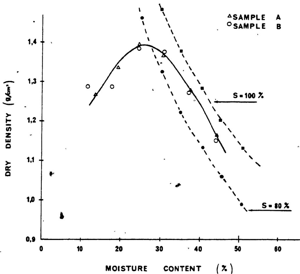
Figure 5.3 Observed compaction curve of the clay soil by the standard Proctor test.
