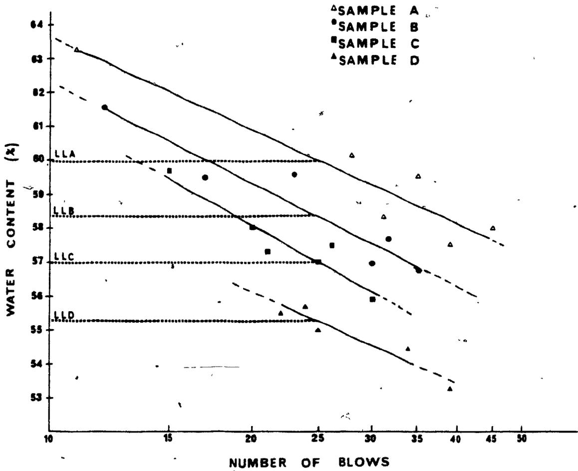
Figure 5.2 Observed critical moistures for liquid limit (LL) test.
