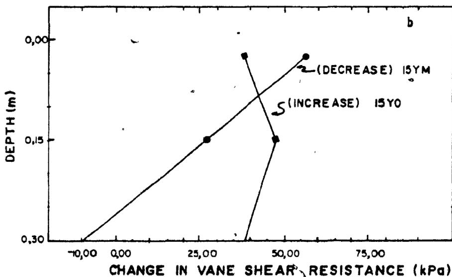
Figure 5.12 Observed changes in vane shear resistance profiles due to traffic and tillage treatments.
