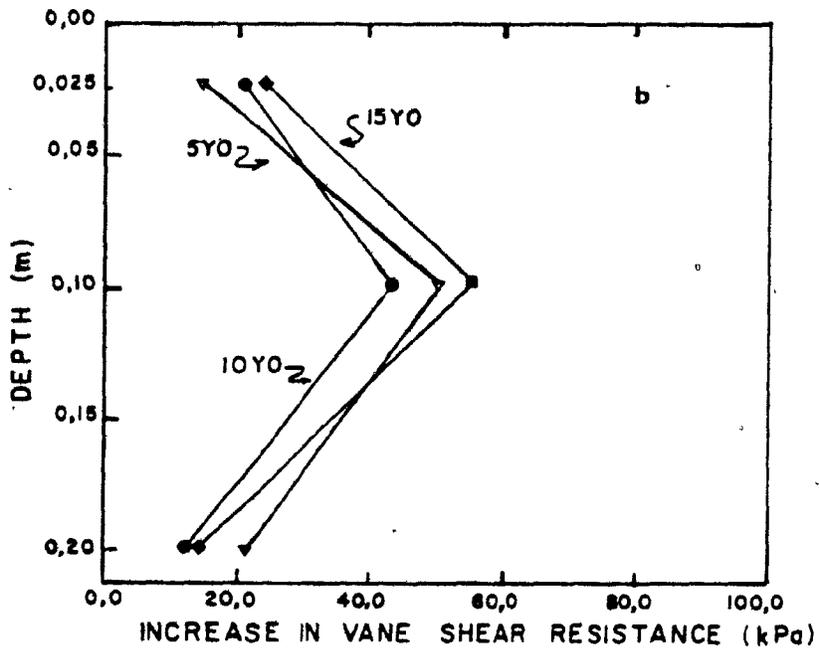
Figure 5.11 Observed changes in vane shear resistance profiles due to traffic treatments.
