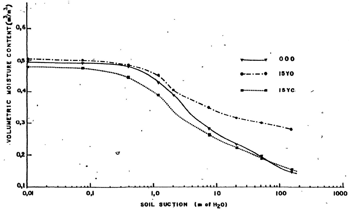
Figure 5.20 Soil moisture retention characteristics at 0,25m depth.
