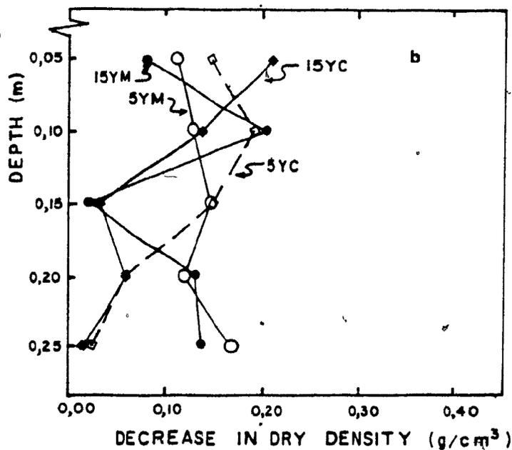
Figure 5.7 Observed changes in dry density profiles due to tillage treatments.
