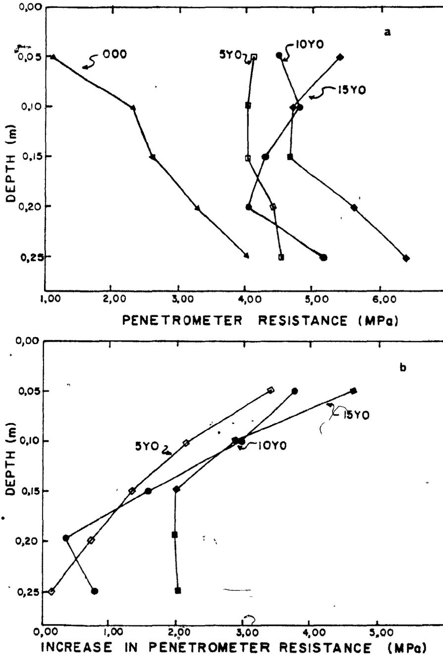
Figure 5.8 Observed changes in penetrometer resistance profiles due to traffic treatments.
