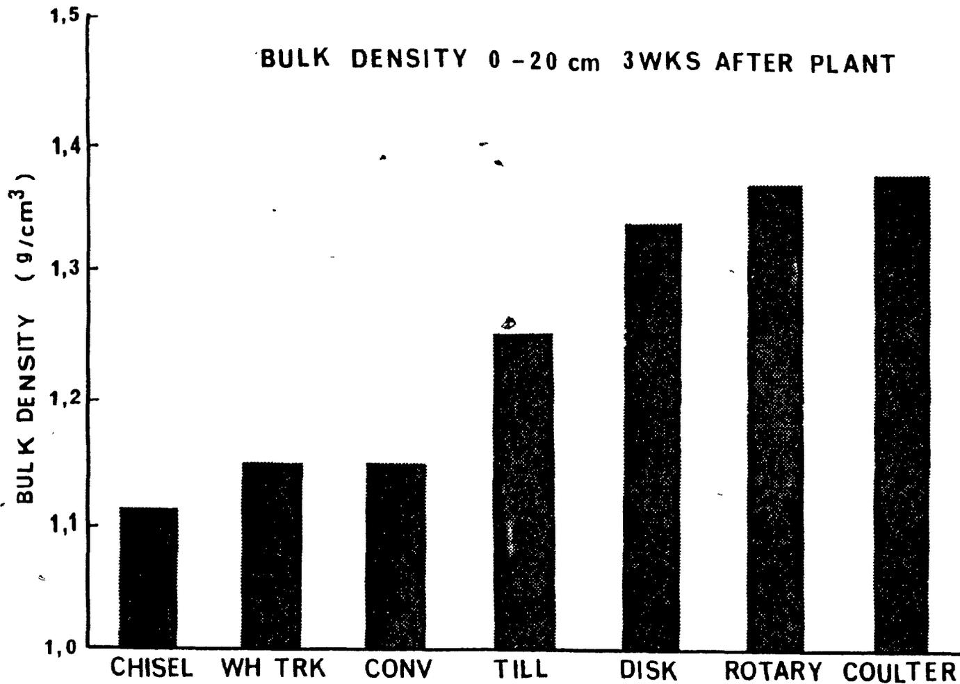
Figure 2.7 Change of bulk density due to different tillage treatments (redrawn from Mannering et al., 1975).
