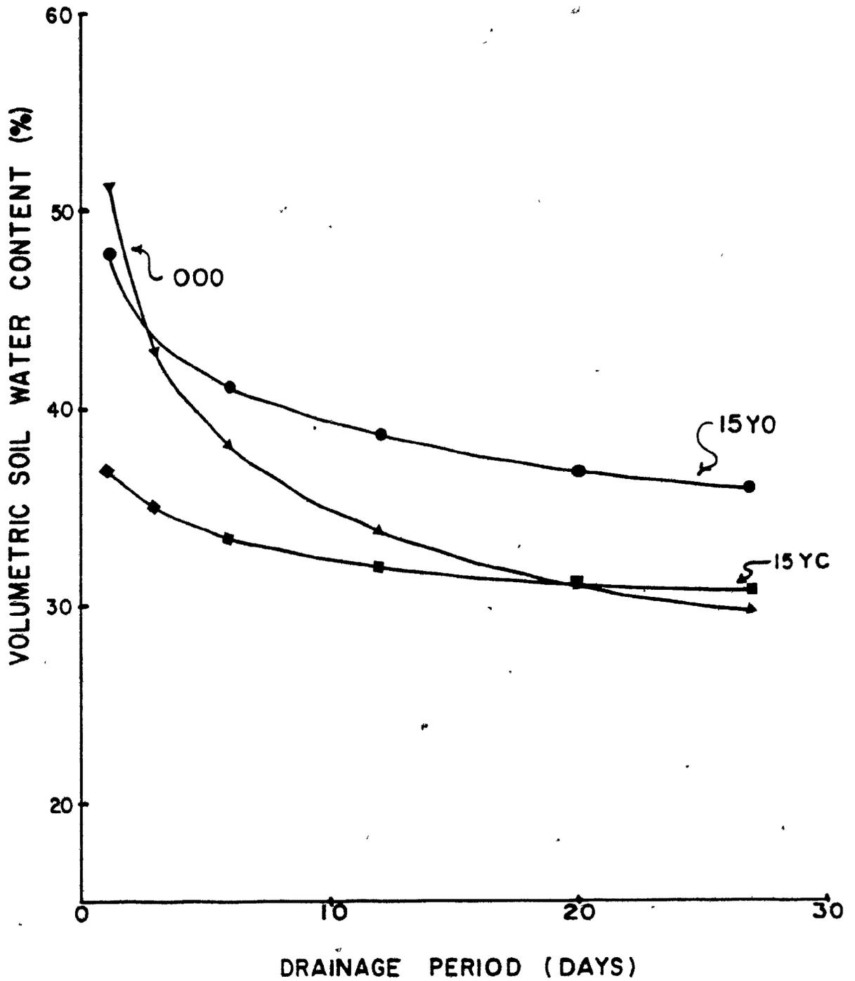
Figure 5.17 Volumetric moisture content versus drainage period at 0,15m depth.
