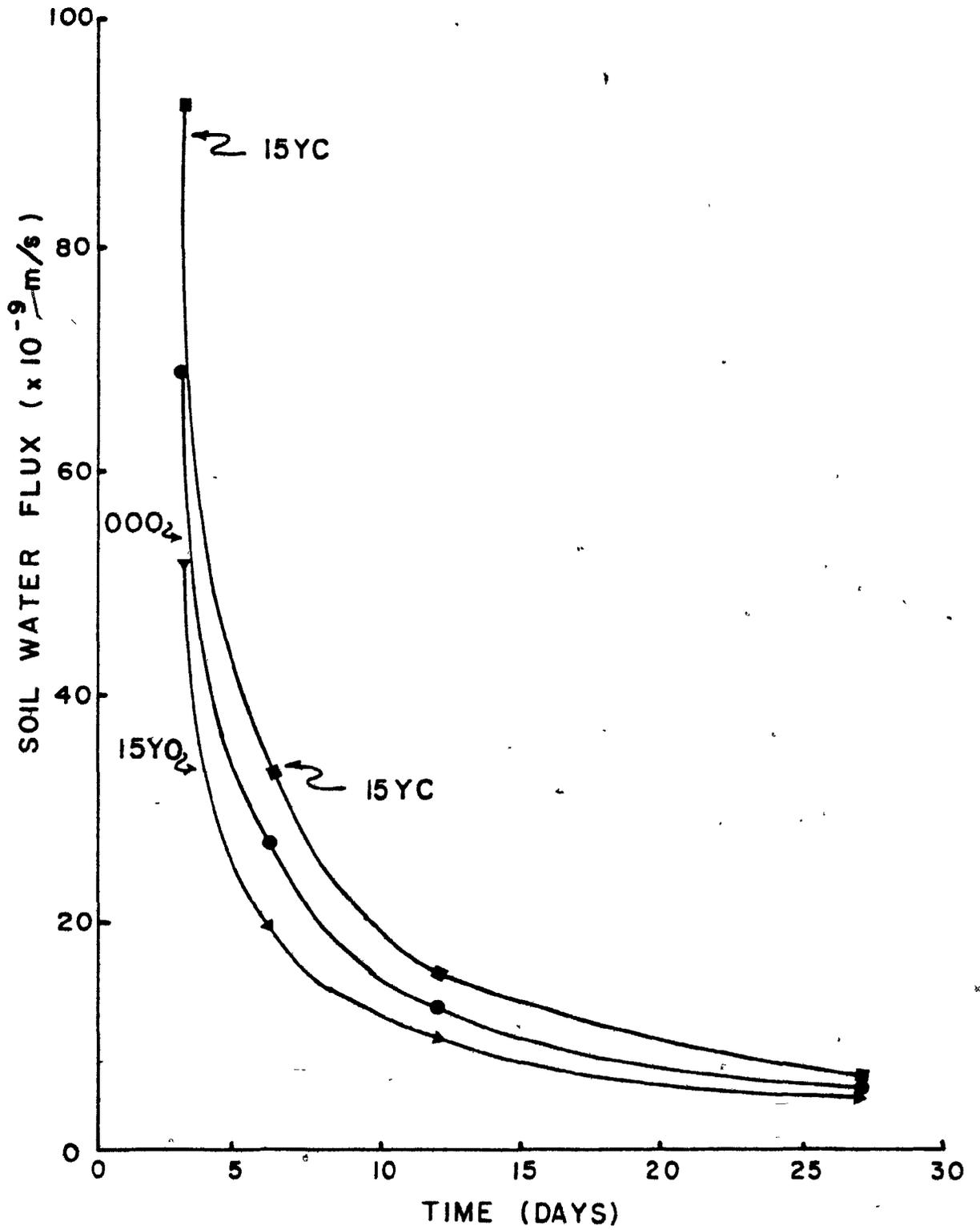
Figure 5.19 Soil water flux leaving 0,25m profile.
