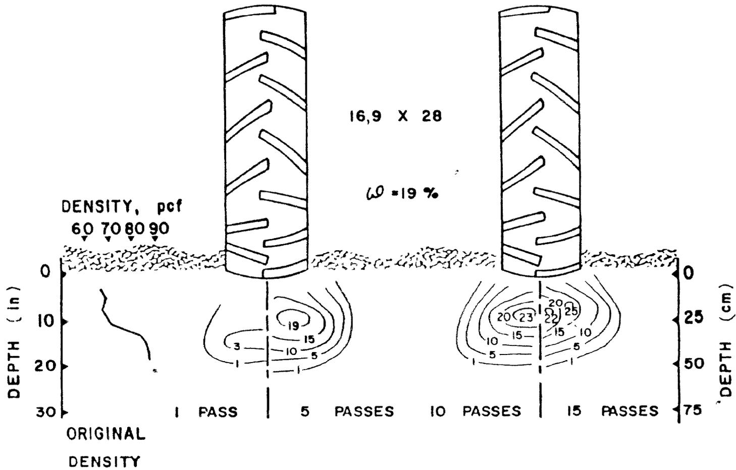
Figure 2.2 Contours of dry density increase due to tractor tire (42,9 x 71,1cm) single pass and multiple passes (after McKyes et al., 1975).
