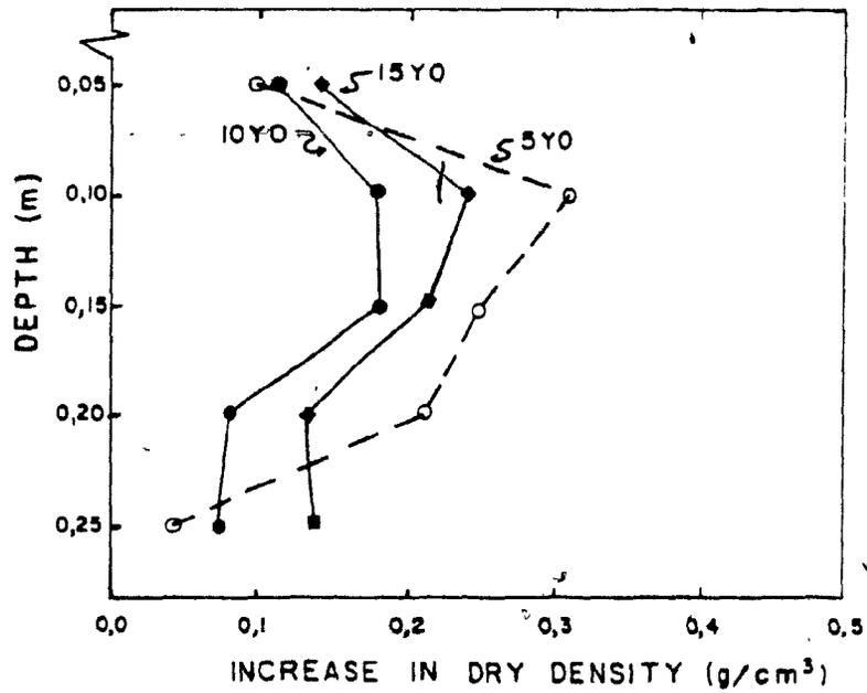
Figure 5.4 Observed changes in dry density profiles due to traffic treatments.
