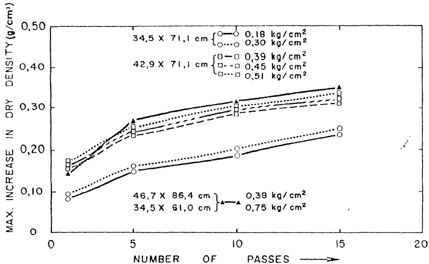
Figure 2.3 Effect of increase in number of passes on compaction for different tires (after Raghavan et al , 1977b)
