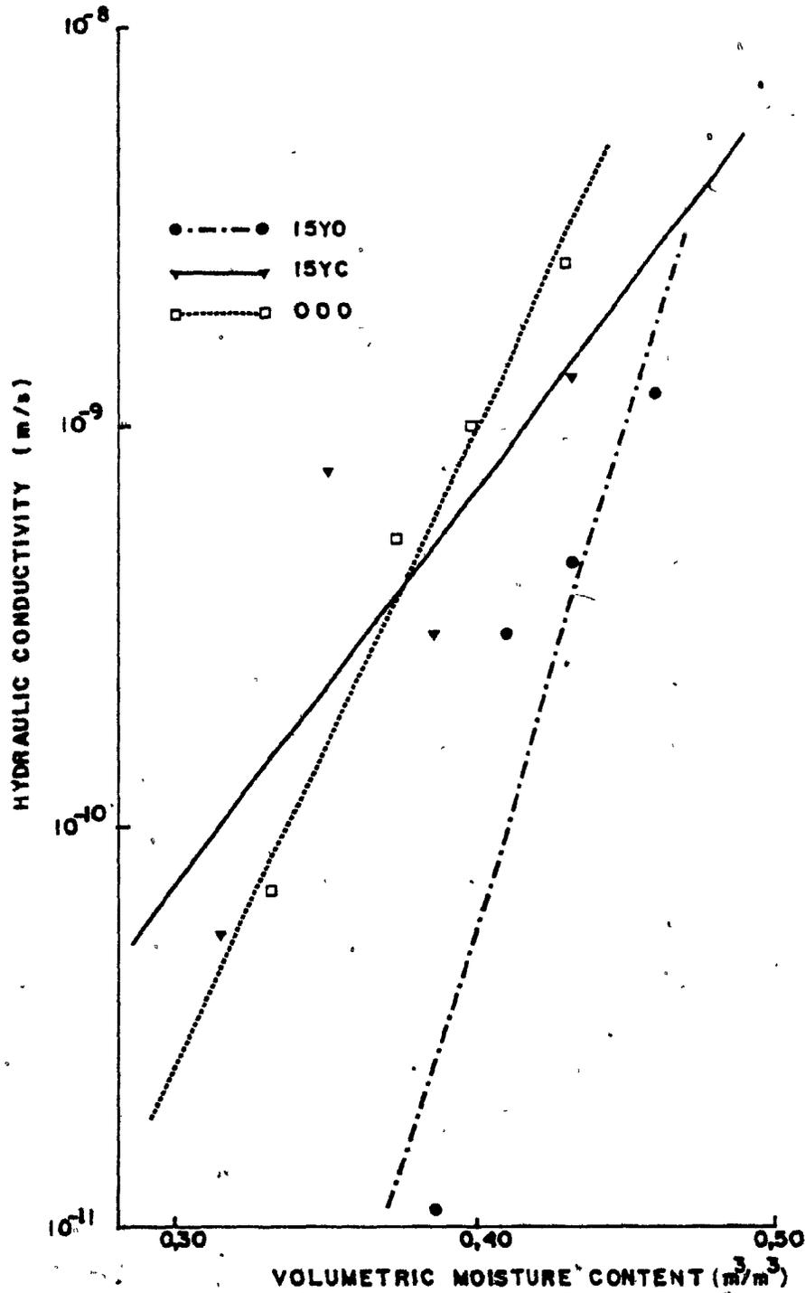
Figure 5:21 Effect of compaction and tillage treatments on unsaturated hydraulic conductivity of the soil at 0,25m depth.
