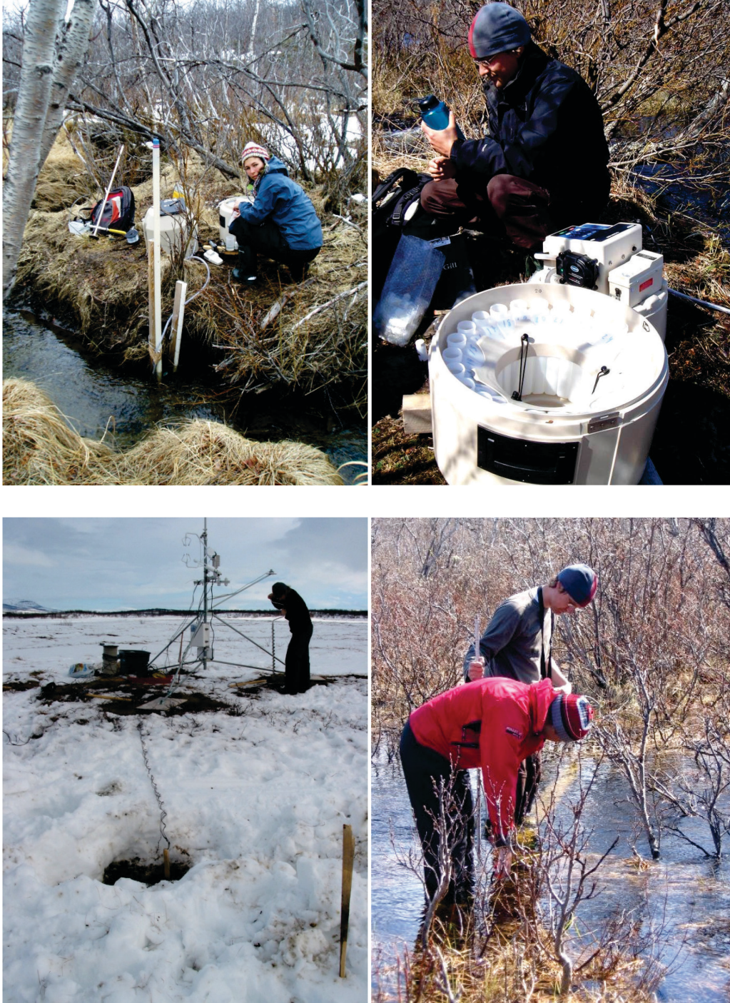
Figure 1.3. Instrumentation and fieldwork in Stordalen catchment. Stream sampling site installed with auto-sampler, water table sensor, electrical conductivity and temperature sensors (Top left). Emptying the auto-sampler after storm event (Top right). Installing the micrometeorological tower at Stordalen (Bottom left). Measuring discharge during peak snowmelt runoff (Bottom right).
