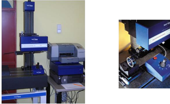
Figure 3-12: The 3D surface scanner Taylor Hobson Talysurf 120 with a close up on the scanning process.
